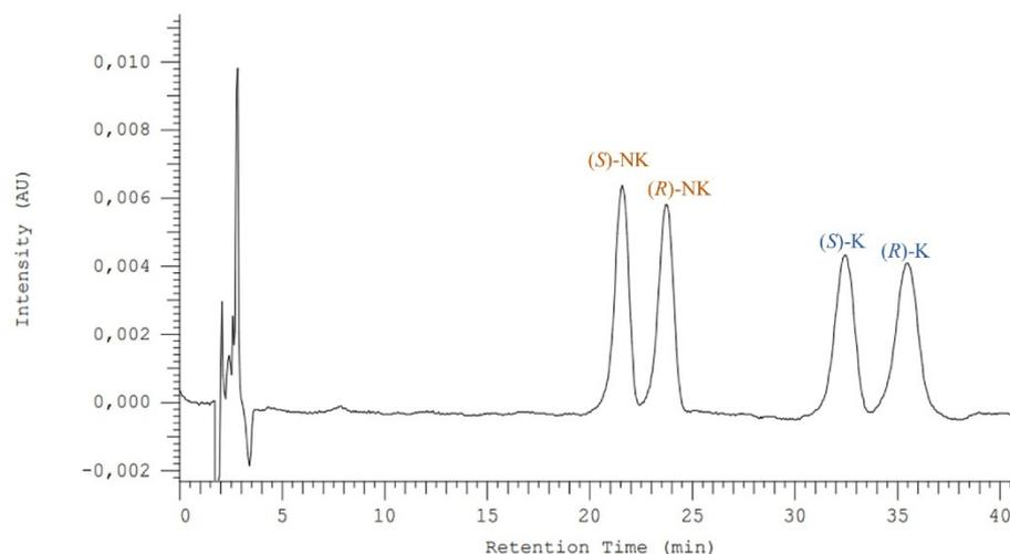
**Figure 2.** Chromatogram of enantioseparation of K and NK (50  $\mu\text{g/mL}$  in MeOH) in the analytical Lux<sup>®</sup> 3  $\mu\text{m}$  Cellulose-4 column by LC-DAD at RT. Mobile phase: 20 mM ammonium acetate in UPW (0.1% DEA) and ACN (75:25,  $v/v$ ); flow-rate: 1 mL/min; injection volume: 10  $\mu\text{L}$ ; detector: 220 nm.
