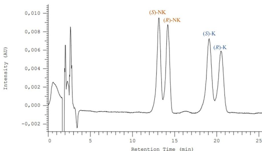
**Figure 3.** Chromatogram of the enantioseparation of K and NK (at 50  $\mu\text{g/mL}$  in MeOH) in the analytical Lux<sup>®</sup> 3  $\mu\text{m}$  Cellulose-4 column by LC-DAD at room temperature. Mobile phase: 20 mM ammonium acetate in UPW (0.1% DEA) and ACN (70:30,  $v/v$ ); flow rate: 1 mL/min; injection volume: 10  $\mu\text{L}$ ; detection: 220 nm.
