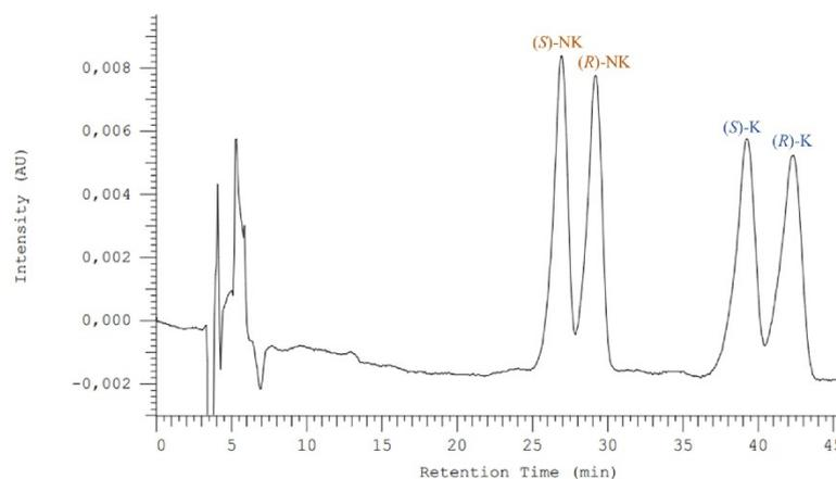
**Figure 1.** Chromatogram of enantioseparation optimization of K and NK (at 50  $\mu$ g/mL in MeOH) in the analytical Lux<sup>®</sup> 3  $\mu$ m Cellulose-4 column by LC-DAD at RT. Mobile phase: 20 mM ammonium acetate in UPW (with 0.1% of DEA) and ACN (70:30, v/v); flow rate: 0.5 mL/min; injection volume: 10  $\mu$ L; detection: 220 nm.
