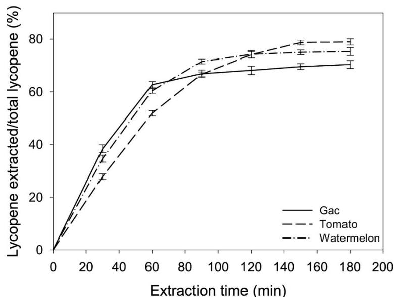
**Figure 8.** Supercritical CO<sub>2</sub> extraction yield over time for three fruits (gac, tomato and watermelon). Reproduced from [81].
