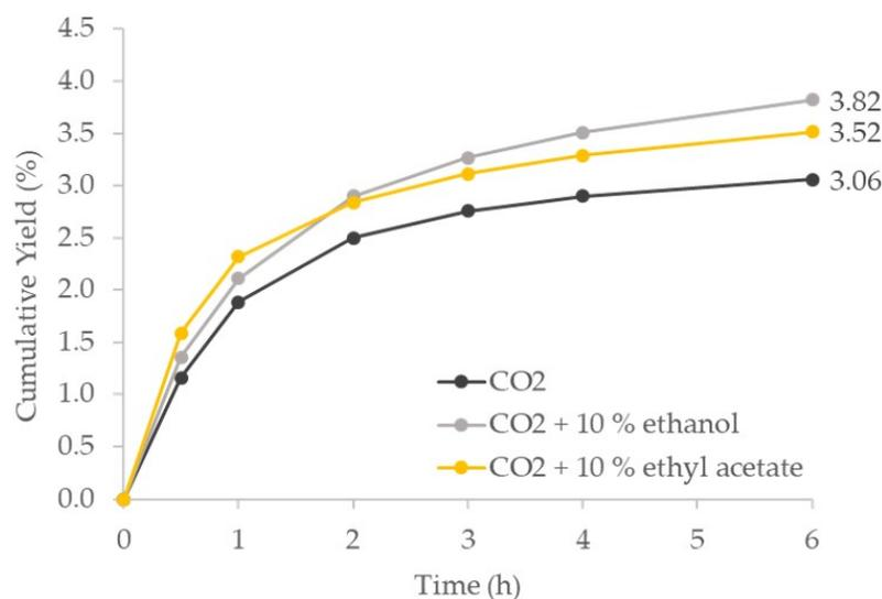
**Figure 6.** Extraction curves of tomato pomace using pure CO<sub>2</sub>, CO<sub>2</sub> with 10% ethanol and CO<sub>2</sub> with 10% ethyl acetate at 300 bar/60 °C/12 g/min CO<sub>2</sub>/6 h with no particle size reduction.
