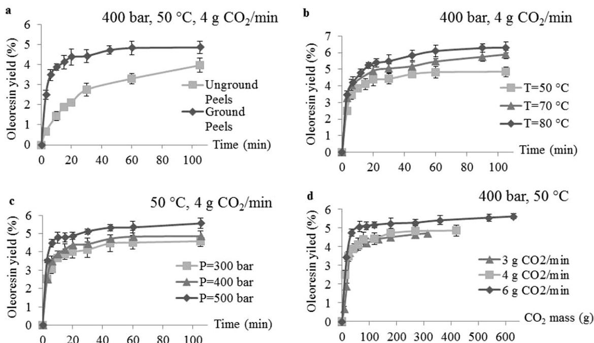
**Figure 4.** SFE curves (yield vs. time) of tomato peels (10 g) with SC-CO<sub>2</sub> to illustrate the effect of (a) particle size, (b) temperature, (c) pressure, and (d) flow rate. Reproduced from [79].
