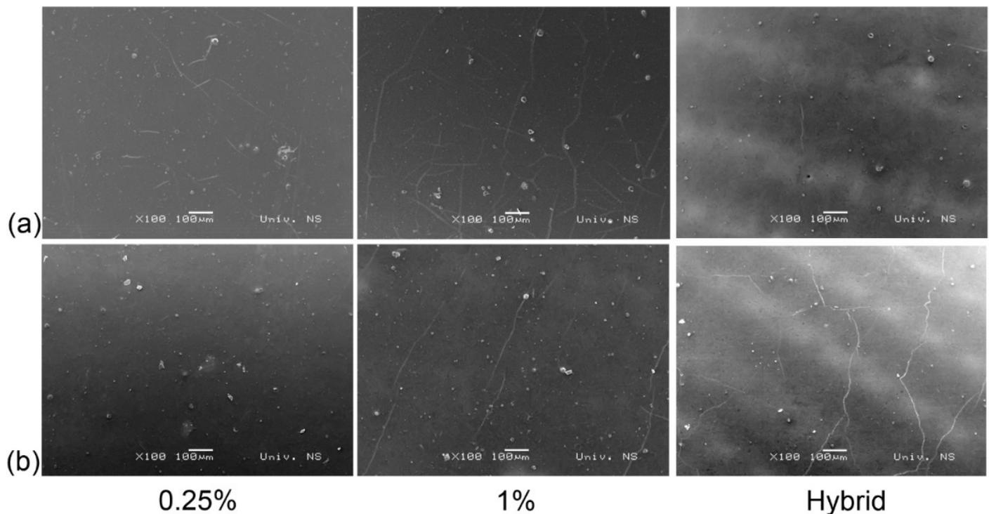
**Figure 2.** SEM micrographs of samples coated by nanocomposite containing (a) ZnO and (b) TiO<sub>2</sub>.
