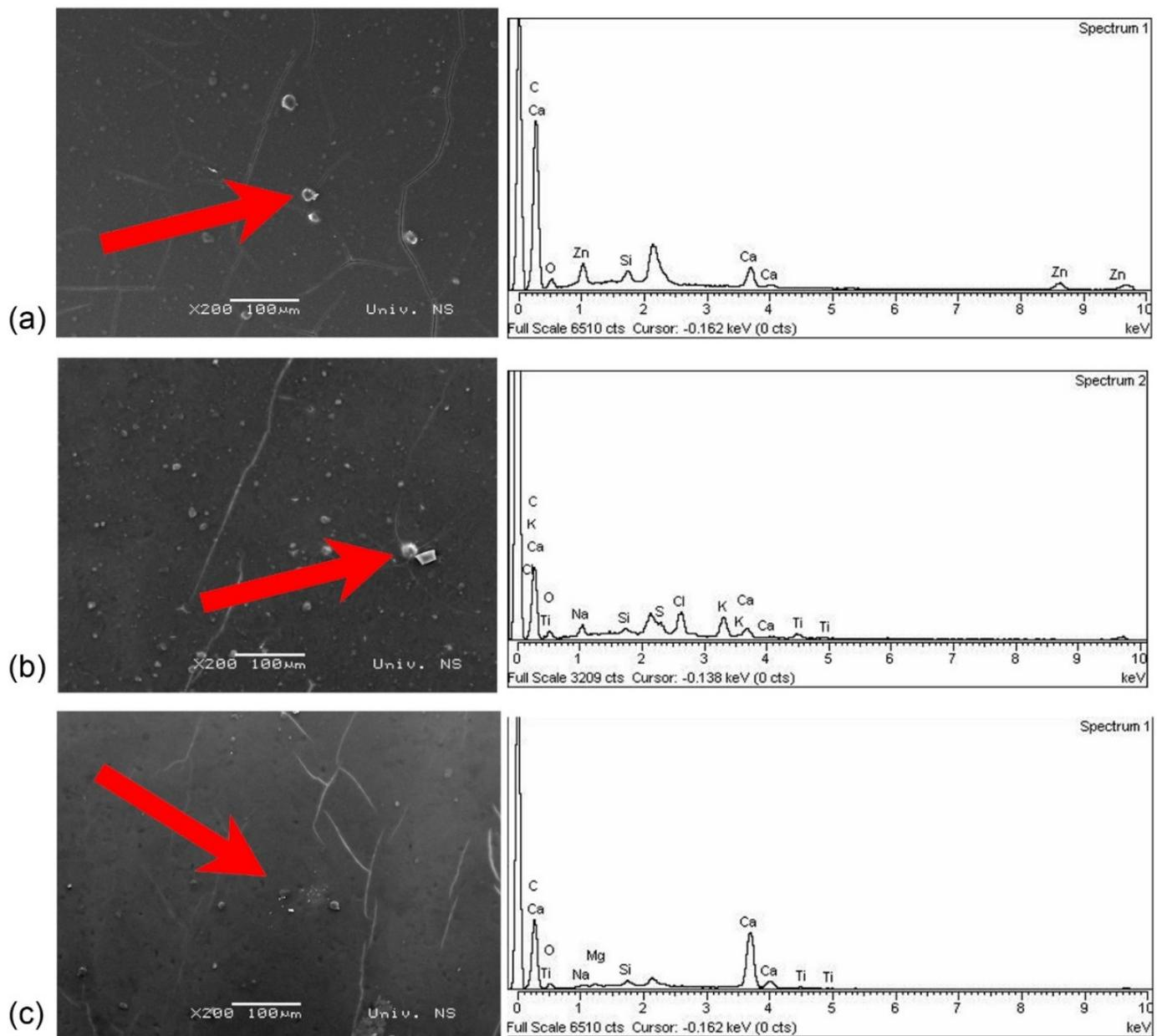
**Figure 3.** Position on the micrograph (red arrow) and EDS spectra on the samples: (a) 1% ZnO nanoclusters, (b) 1% TiO<sub>2</sub> nanoclusters, (c) 1% TiO<sub>2</sub>/SiO<sub>2</sub> nanoclusters.
