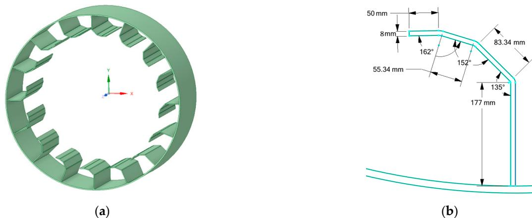
**Figure 1.** The geometrical characteristics of the real model used in the analysis: (a) flights' arrangement inside the drum, (b) the shape and dimensions of the flights.
