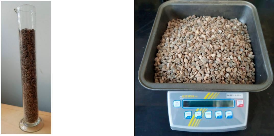
**Figure 4.** Determination of bulk particle density.
