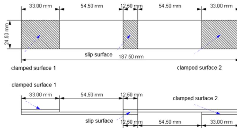
**Figure 3.** The size of the tested samples made of G11 glass epoxy sheets.
