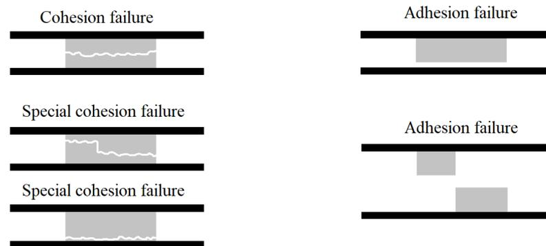
**Figure 2.** Adhesive and cohesive joint failures acc. to EN ISO 10365:1992. (The figure was modified according to [10]).
