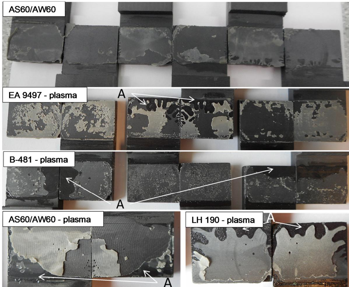
**Figure 9.** Images of broken joints tested at 130 °C for each type of adhesive. Areas which do not have enough adhesive are marked as A.
