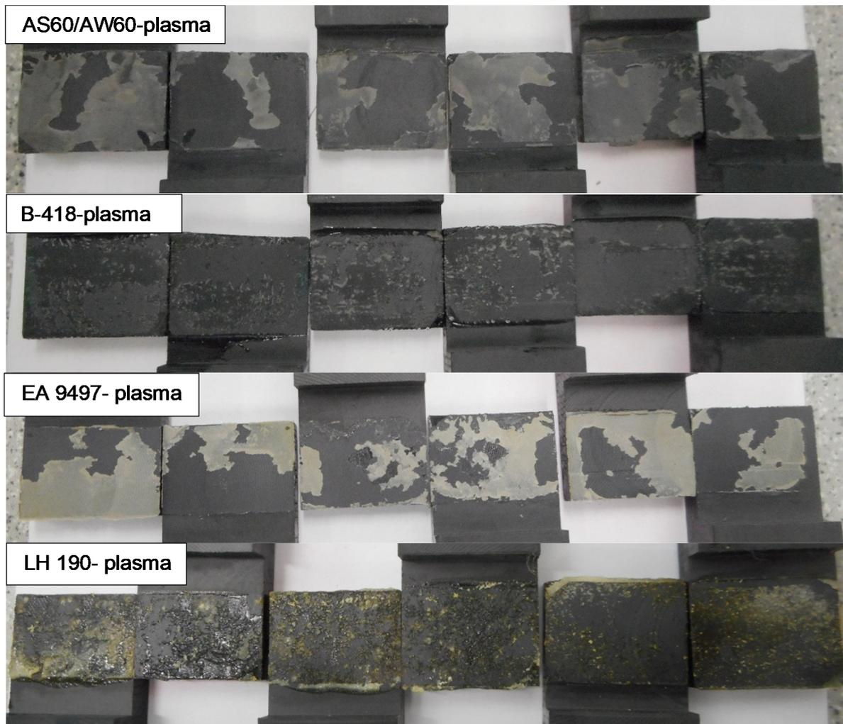
**Figure 10.** Images of broken adhesive joints of PPS-40GF composites tested at 180 °C.
