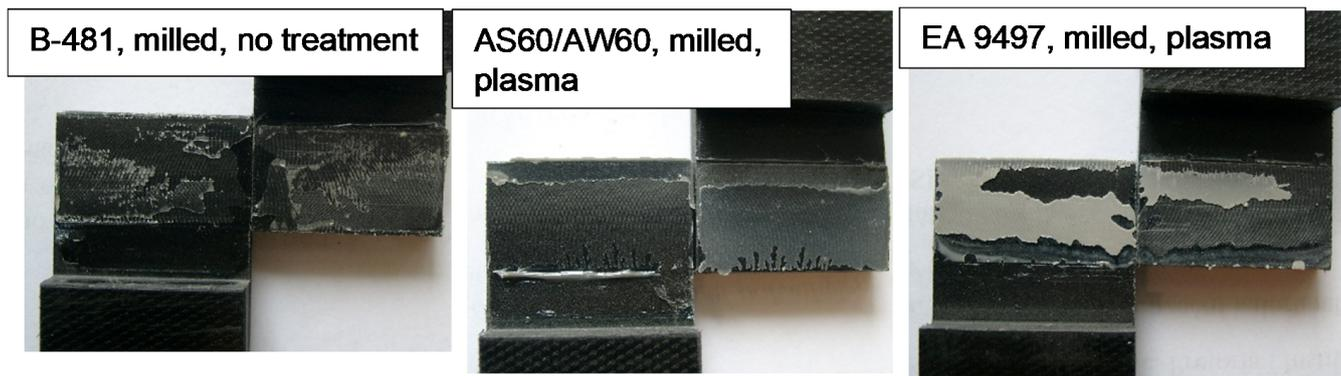
**Figure 7.** Photos of PA66-GF30 samples fracture, tests at 110 °C.
