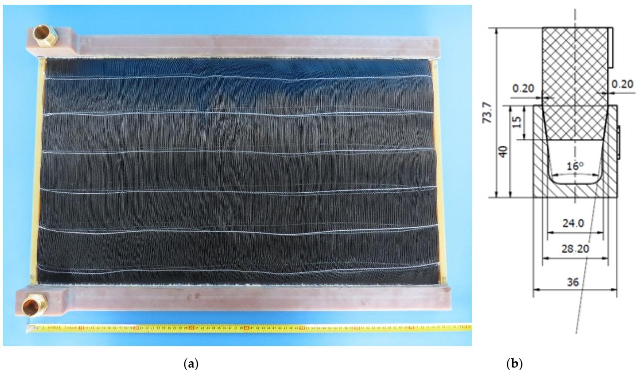
**Figure 1.** (a) Plastic heat exchanger with coolant manifolds made of glass fabric enforced epoxy G11 EPGC308, adopted from [1]; (b) diagram of the bonding connection applied to glue the heat exchanger core to the manifolds.
