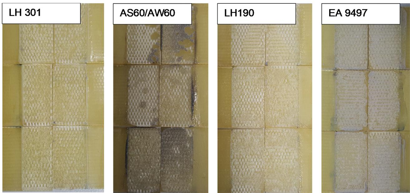
**Figure 6.** Fracture surfaces of the 4 best-performing adhesives—130 °C test. The slip surfaces of all the adhesives show the presence of the adhesive on both sides of the samples which can be interpreted as cohesive failure. However, in all cases, the majority of the adhesive layers were on one side, showing the nature of the adhesive failure nature.
