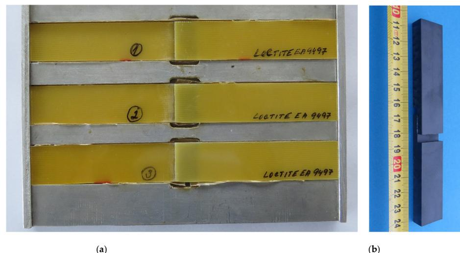
**Figure 4.** (a) Aluminum frame with glass epoxy samples; (b) milled PA66-GF30 sample.
