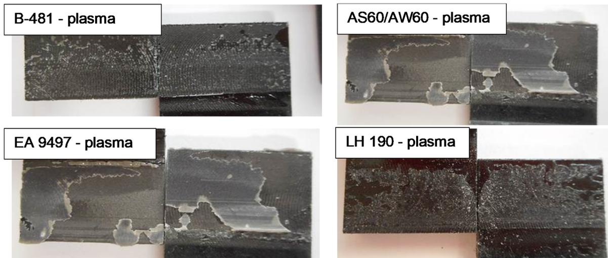
**Figure 8.** Photos of PA66-GF30 samples fracture, tests at 160 °C.
