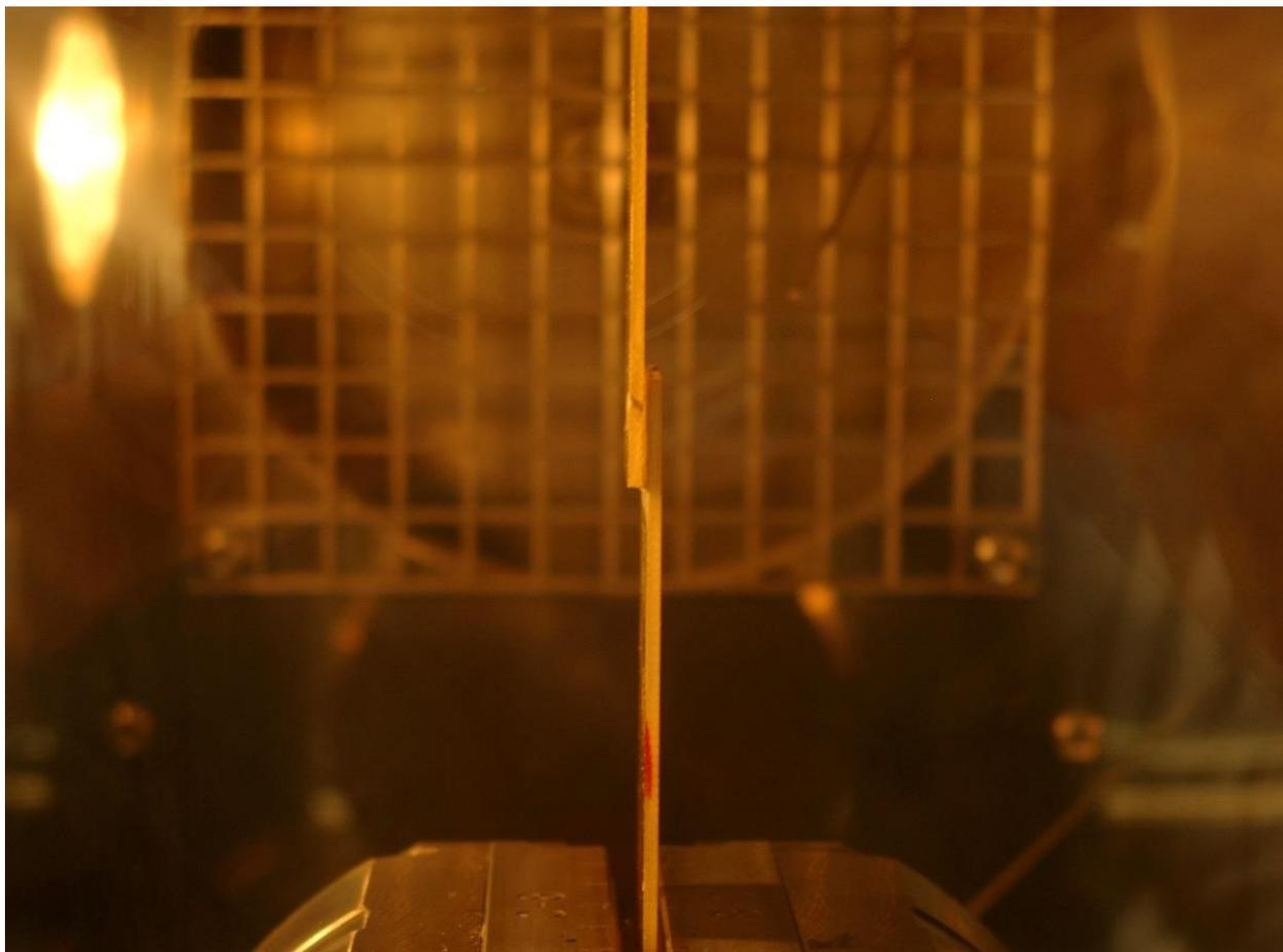
**Figure 5.** Epoxy sheet sample fixed in the clamping jaws of the heated chamber of the tensile machine Z010 TE, Zwick & Roell.
