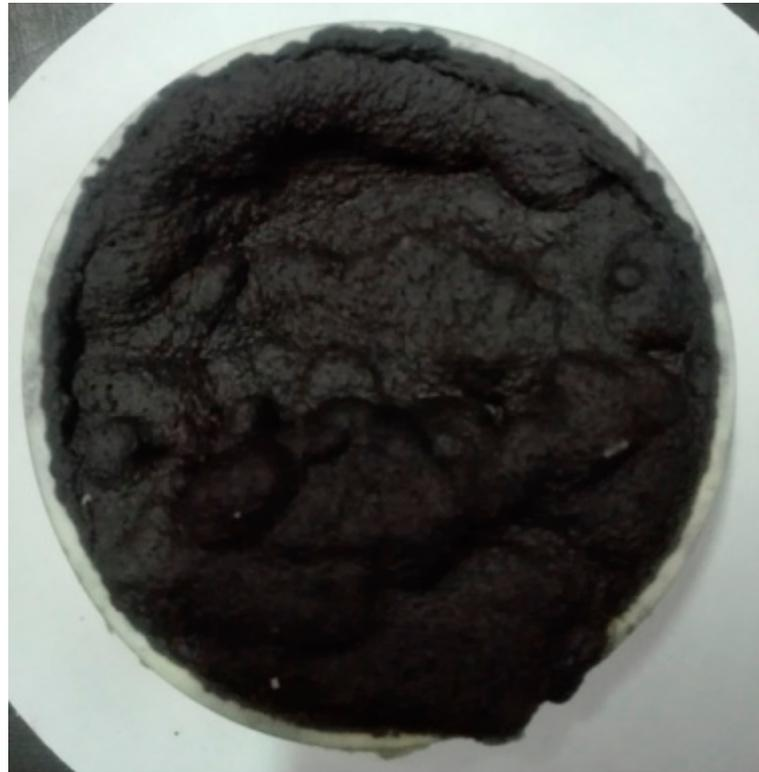
**Figure 1.** SCC after alkali fusion treatment.
