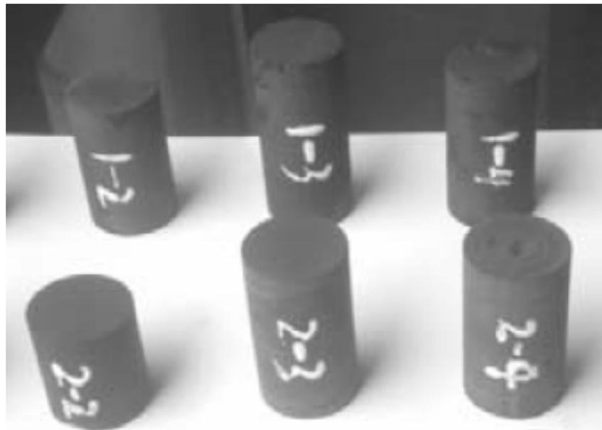
**Figure 5.** Processed core samples for the rock mechanical tests.
