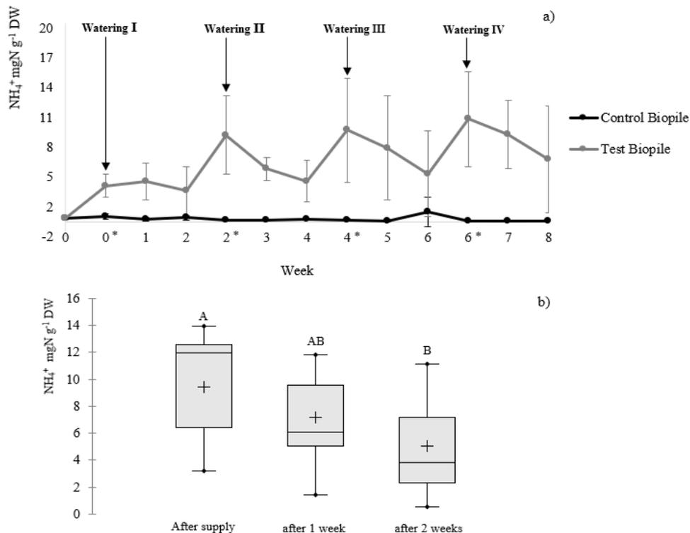
**Figure 2.** (a) Temporal evolution of the ammonium nitrogen ( $\text{NH}_4^+$ ) concentration in the water extracts, and (b) monitoring of the ammonium nitrogen ( $\text{NH}_4^+$ ) abatement evolution in the test biopile (\* means after watering and the error bars represent standard deviations ( $n = 3$ )). Different letters above boxplots indicate a significant difference between plots according to the Kruskal–Wallis test with Dunn’s procedure,  $p$  value = 0.05.
