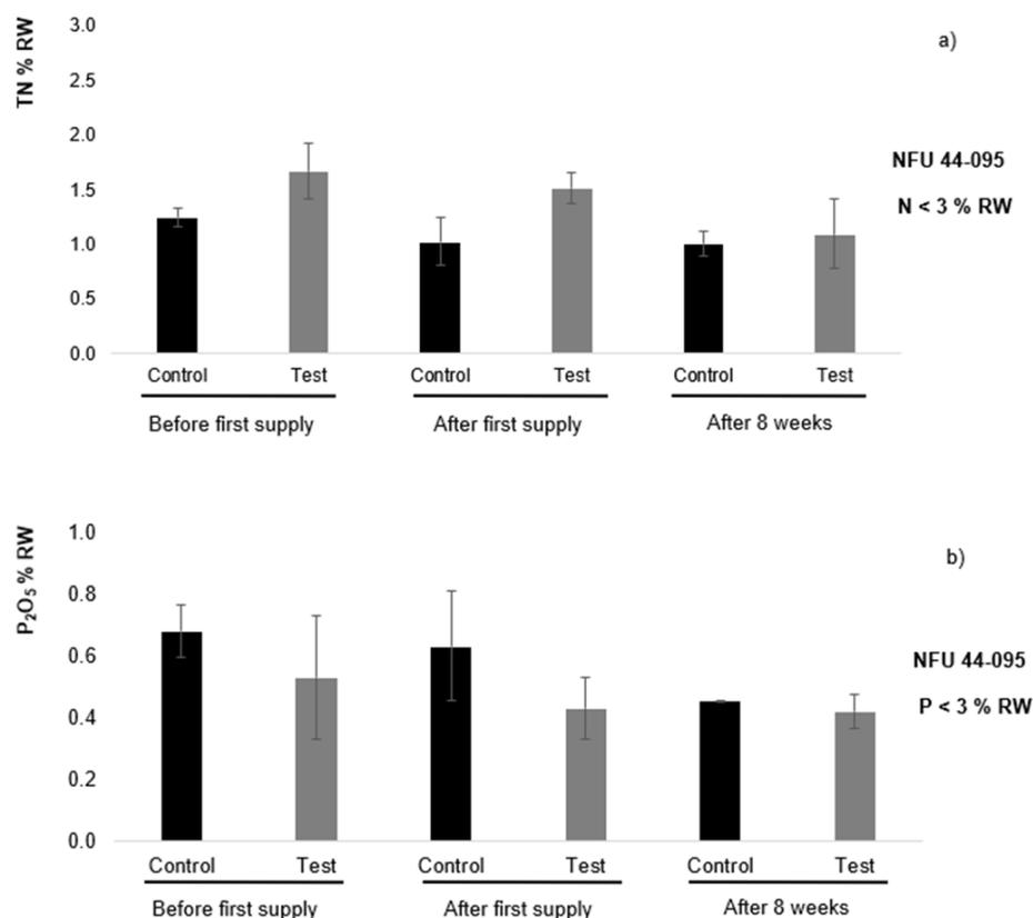
**Figure 6.** The agronomic parameters (a) TN (% RW) and (b) P<sub>2</sub>O<sub>5</sub> (% RW) measured in the two biopiles: Control (biopile watered with clean water) and Test (biopile watered with leachate),  $n = 3$ .
