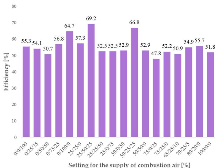
**Figure 3.** The efficiency comparison during different settings for air supply.
