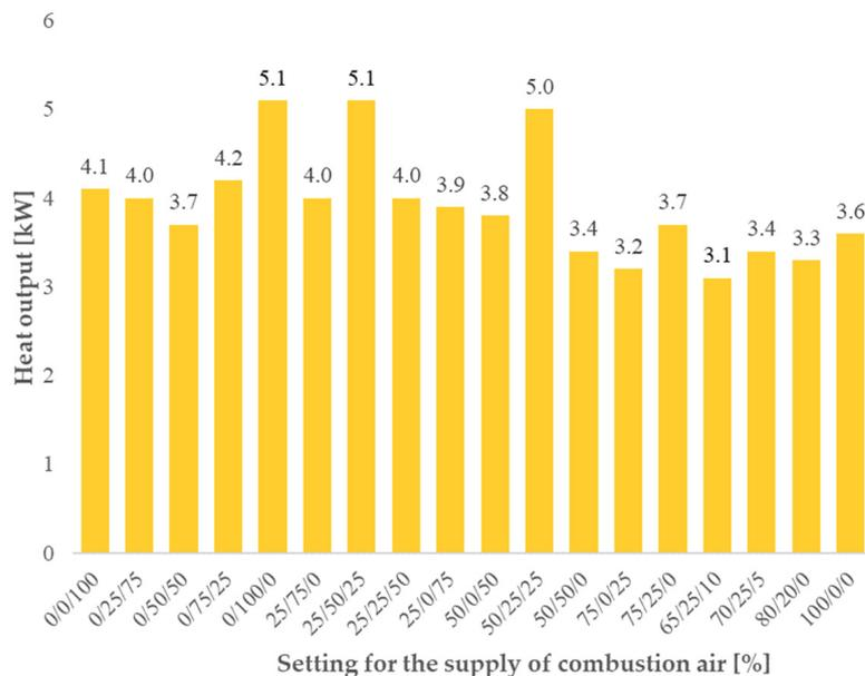
**Figure 4.** The heat output comparison during different settings for air supply.
