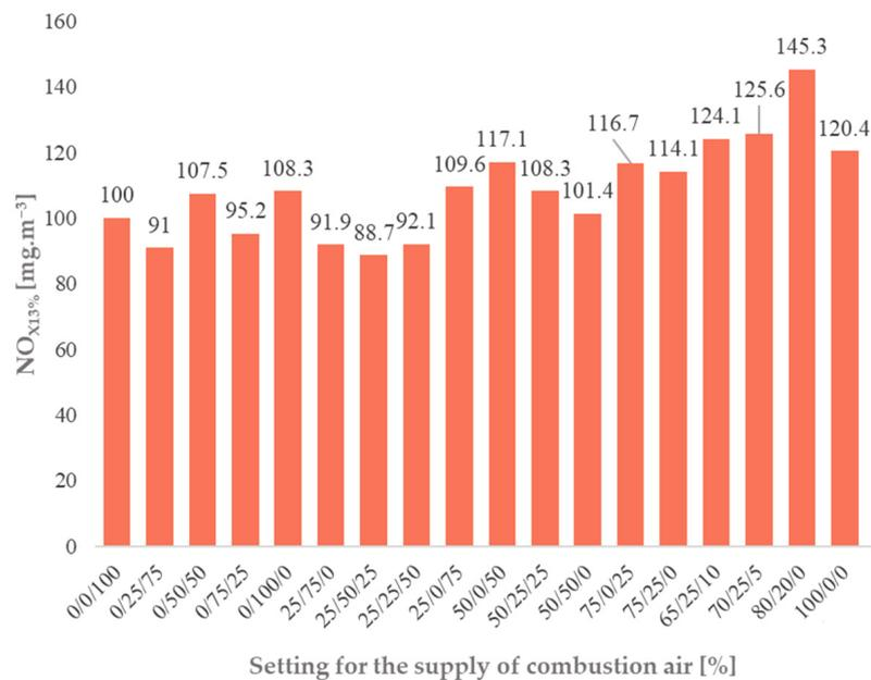
**Figure 6.** The formation of nitrogen oxides during different settings for air supply.
