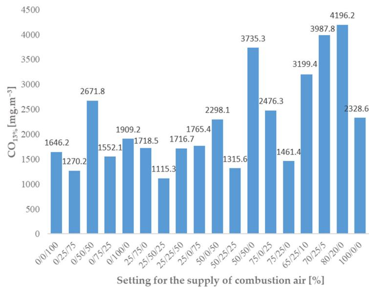
**Figure 5.** The carbon monoxide formation during different settings for air supply.
