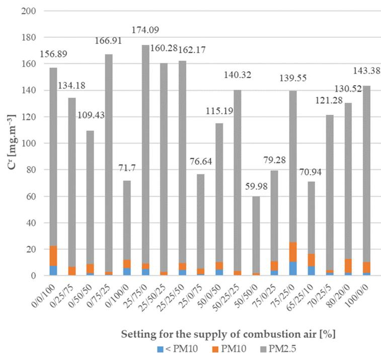
**Figure 7.** The formation of particulate matter during different settings for air supply.
