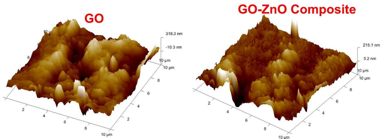
**Figure 4.** AFM image of (i) GO and, (ii) GO-ZnO composite.
