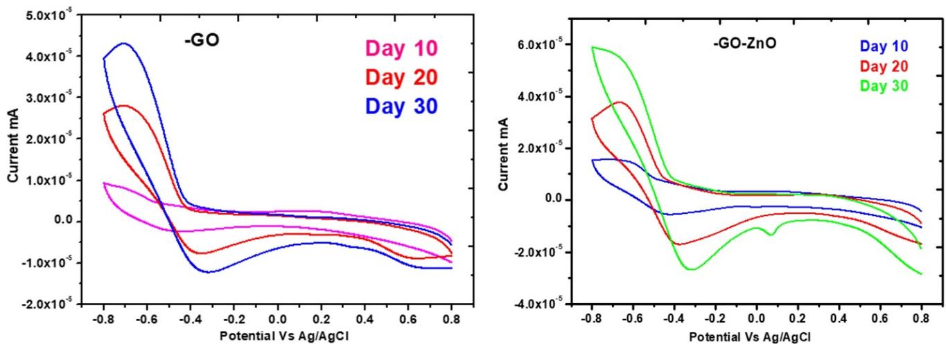
Figure 7. CV study of the GO and GO-ZnO.
