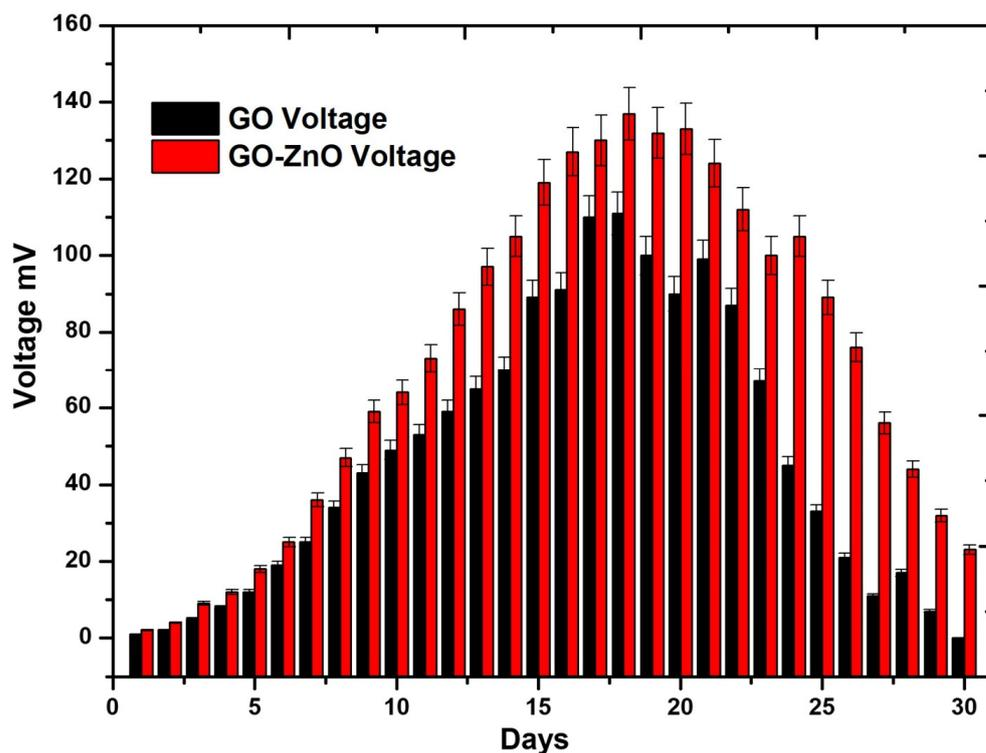
Figure 5. Voltage generation trend through the MFC operation in the presence of self-fabricated anodes.
