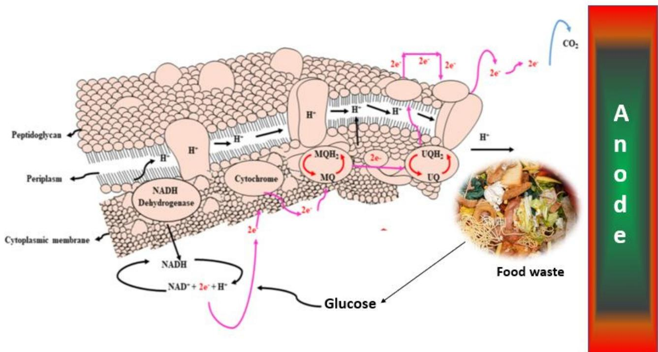
**Figure 9.** Food waste microbiologically oxidized in a single-chamber MFC (figure modified from [64] with Elsevier's permission).
