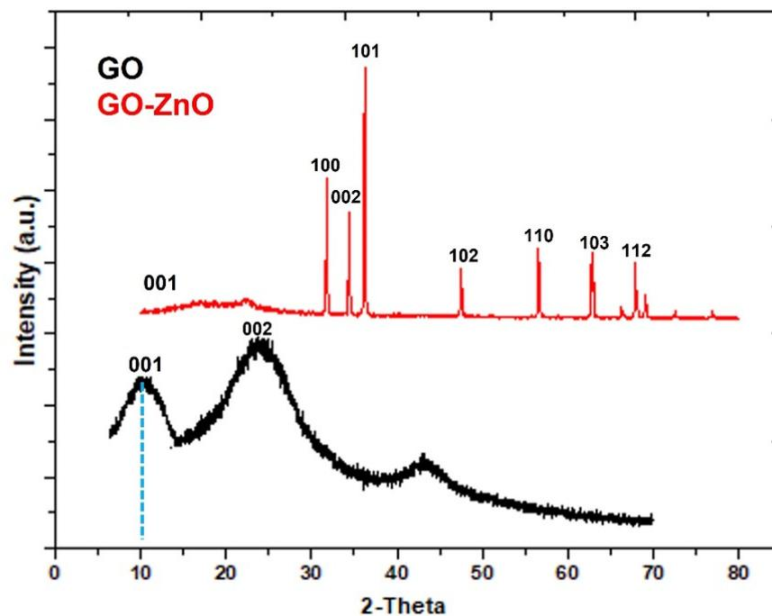
Figure 2. XRD spectra of (i) GO and, (ii) GO-ZnO composite.
