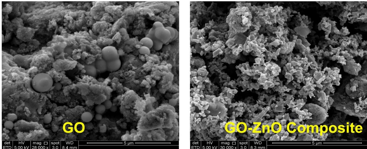
**Figure 3.** SEM analysis of (i) GO and, (ii) GO-ZnO composite.
