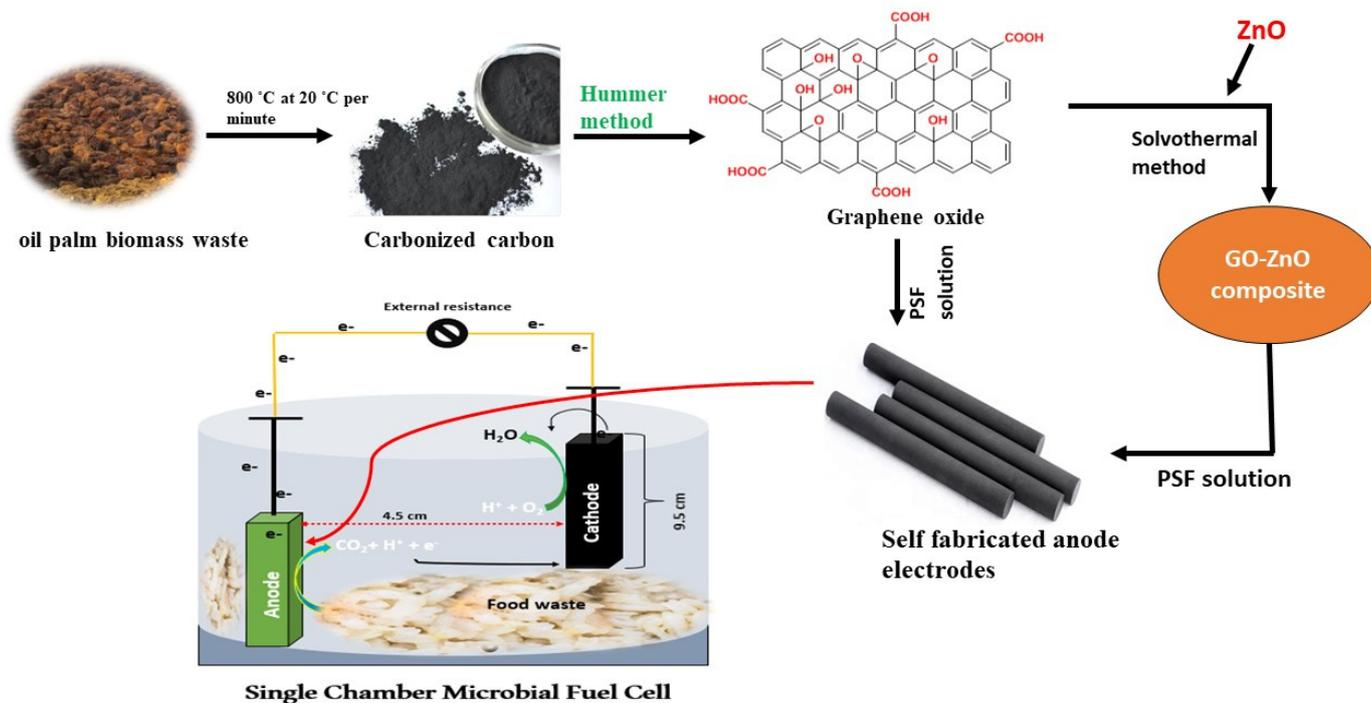
**Scheme 1.** The conversion of oil palm biomass to GO results in the formation of a GO-ZnO composite for the fabrication of anode electrodes for single-chamber MFCs.
