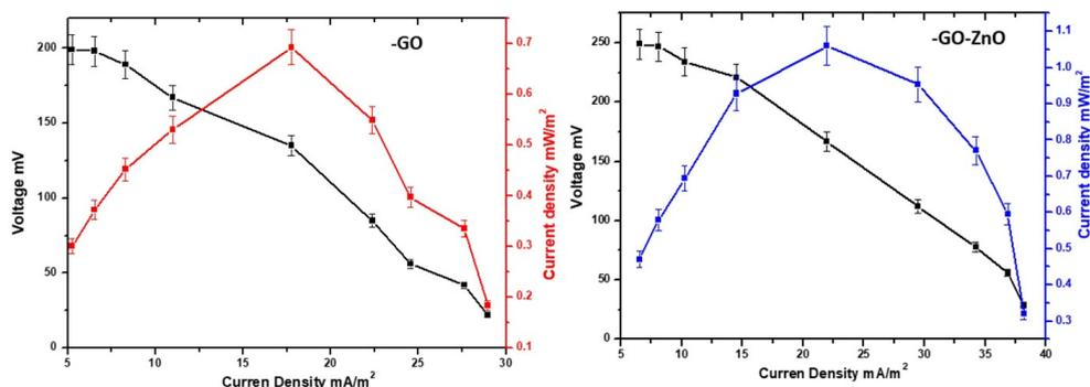
Figure 6. Polarization curves of GO and GO-ZnO anode during the operation.
