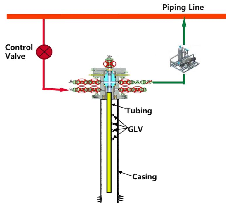
Figure 3. Low pressure wells' gas lift operation loop.
