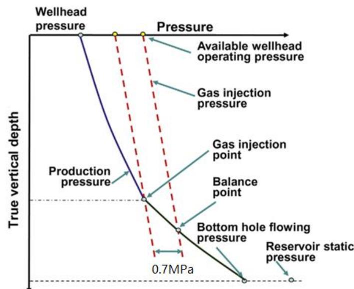
**Figure 8.** Depth of the operating gas injection point.
