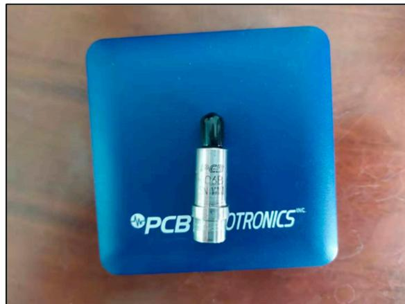
Figure 5. PCB 106b acoustic sensor.
