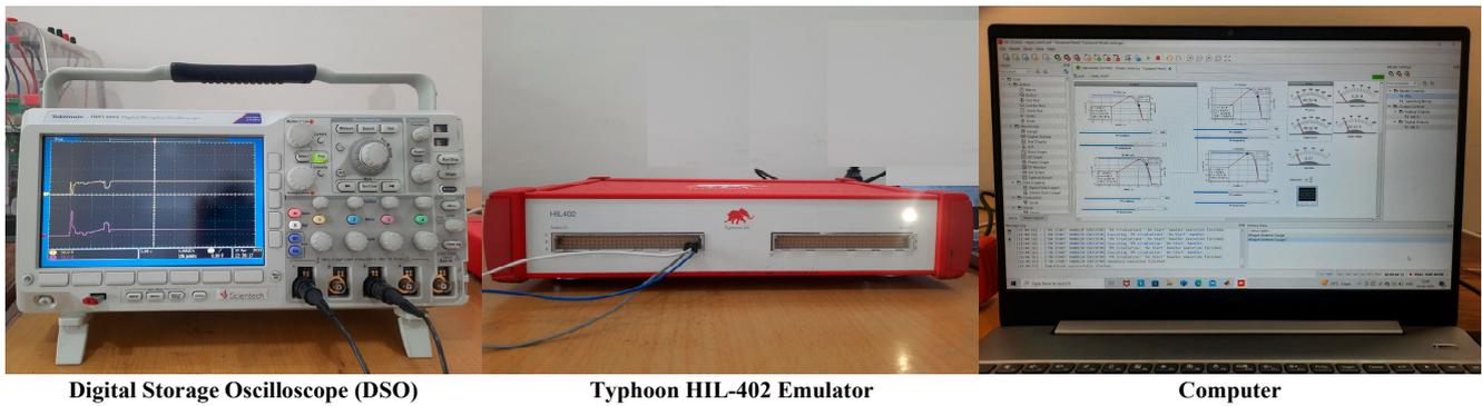
Figure 13. Digital storage oscilloscope (DSO), Typhoon HIL-402 emulator, and host computer.
