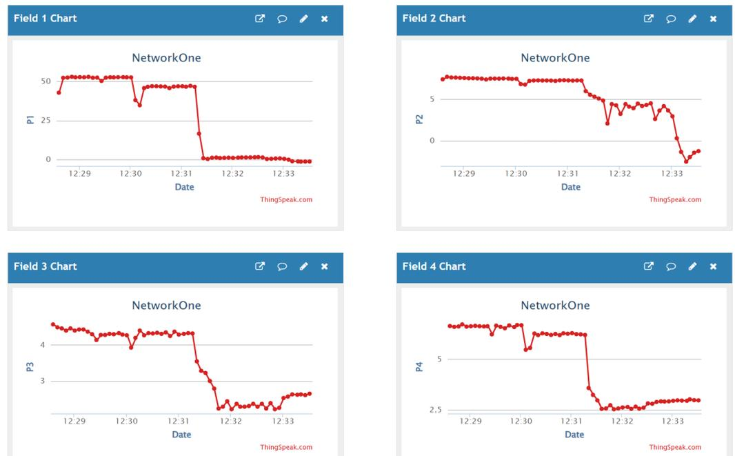
**Figure 7.** Real-time monitoring of the pressure head in the cloud environment (Fields 1 to 4 of the pressure head cloud channel).
