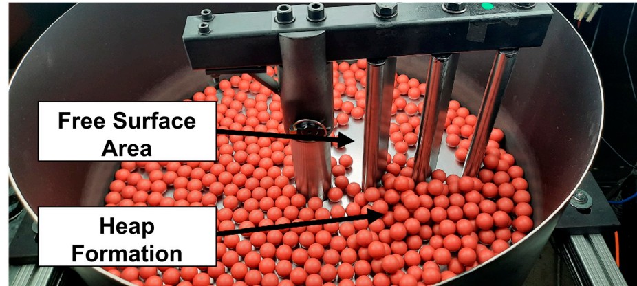
Figure 3. Photograph of the test rig; the black arrows indicate the location of free surface area and the location where heap formation exists (multiple particle layers) [6]. Reproduced with permission from Kriegeskorte et al., Particuology ; published by Elsevier, 2023.
