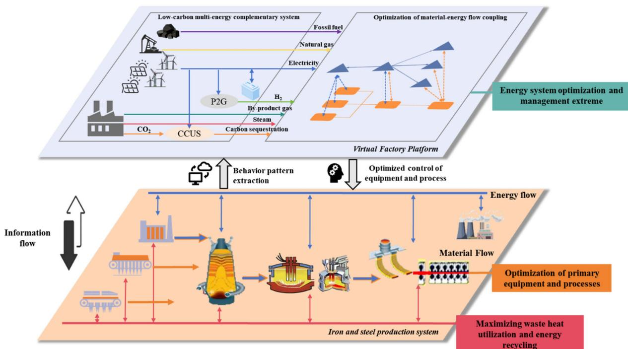
**Figure 4.** Optimization of low carbon steel production system by multi-energy complementary coupling and energy efficiency improvement pathway.
