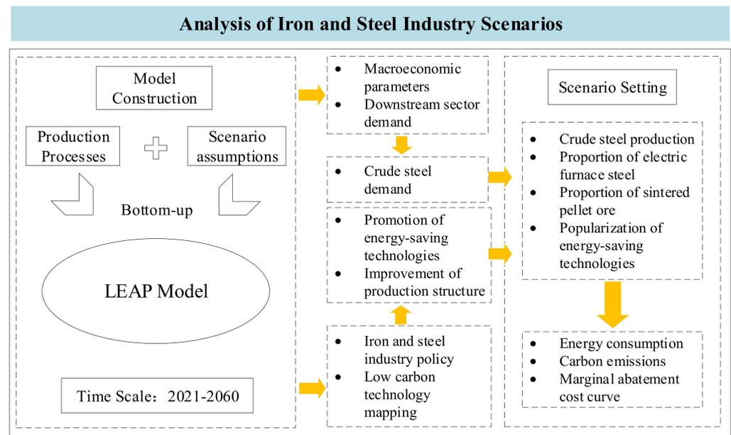
**Figure 6.** Flowchart of carbon emission modeling of the iron and steel industry of China based on the LEAP model.
