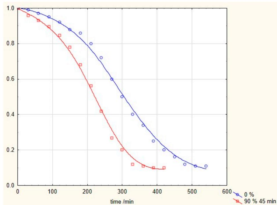
**Figure 2.** Relationship between the moisture ratio and drying time without US and using optimal US processing time, with Weibull model.
