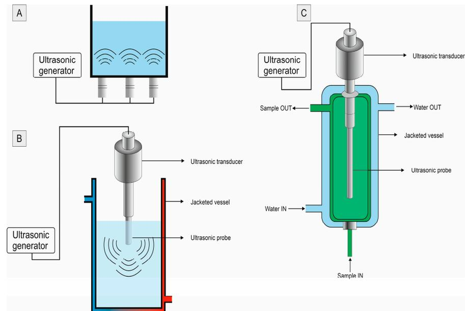
**Figure 1.** Most common ultrasonic setups: (A) bath with probes mounted below: (B) directly immersed probe: (C) continuous flow sonication with cooling.
