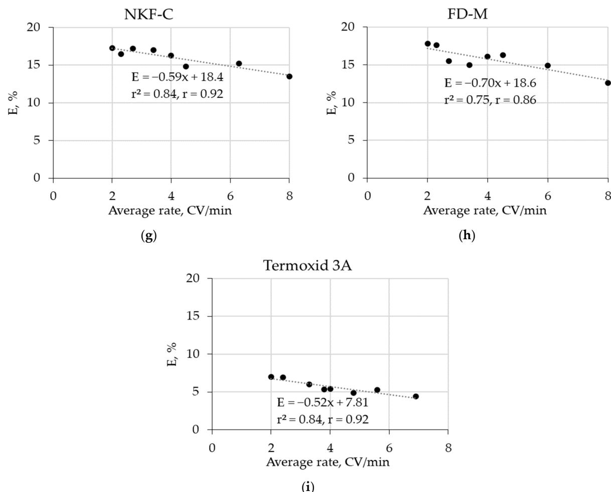
**Figure 2.** Dependence of sorption efficiency ( $E, \%$ ) of  $^{137}\text{Cs}$  on average rate of passage of seawater by sorbents: (a) Niket; (b) Uniket; (c) Termoxid 35; (d) FIC; (e) Anfezh; (f) FSS; (g) NKF-C; (h) FD-M; (i) Termoxid 3A (volume of sorbents—50 mL; the volume of seawater—250 L).
