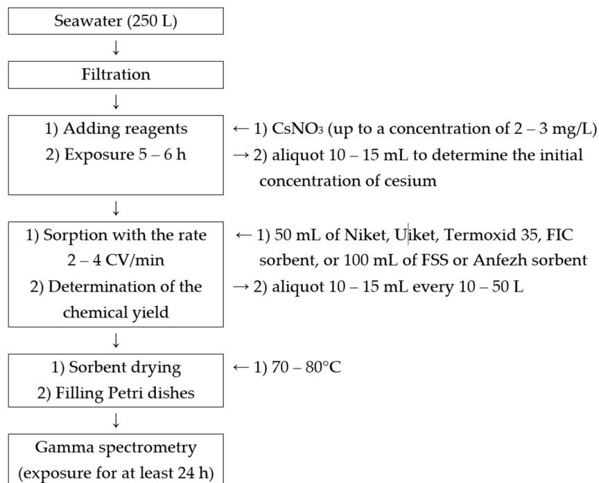
**Figure 3.** Scheme of method developed for  $^{137}\text{Cs}$  sorption.
