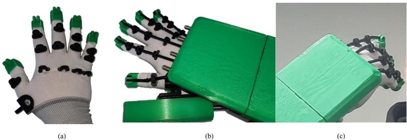
**Figure 13.** Prototype of the wearable glove: (a) glove with fixed exoskeleton frame; (b) fabricated prototype; (c) wearing the prototype and controlling the finger angle.
