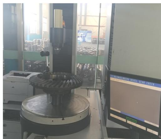
**Figure 4.** Tooth surface errors measuring of gear after heat treatment.
