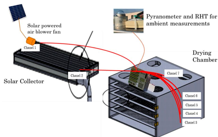
**Figure 1.** Indirect solar dryer for coriander leaves drying process.
