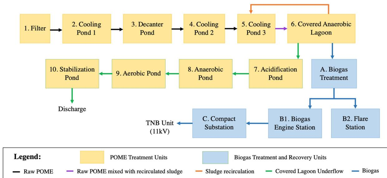
**Figure 2.** Block Diagram of the POME Treatment Process (Adapted from Cheau Chin et al. [15]).
