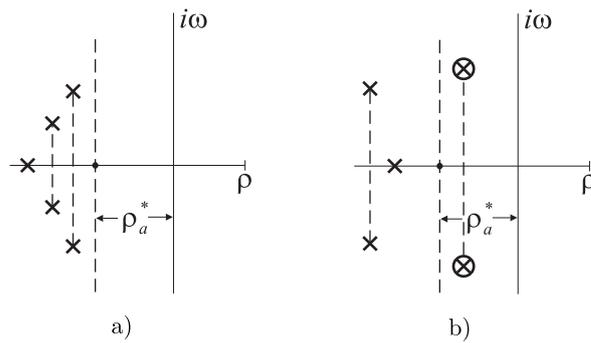
**Figure 2.** The limit of aperiodic stability may (a) or may not (b) coincide with the maximum stability.
