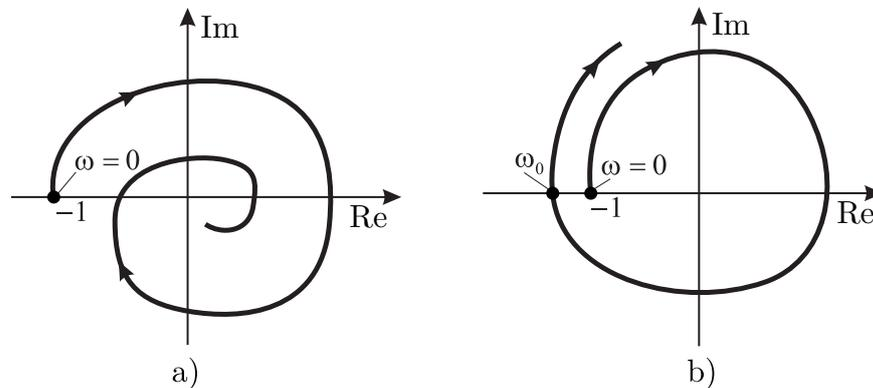
**Figure 3.** The Nyquist plot of the extended response of an open-loop system for cases where the maximum degree of stability is aperiodic (a) and oscillatory (b).
