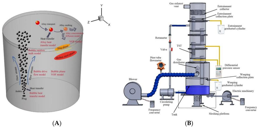
**Figure 4.** (A) Diagram of the simulation model applied to the argon-stirred ladle [6]. (B) Experimental setup used by Tao et al. to investigate the hydrodynamic performance of a countercurrent total spray tray under sloshing conditions [7].
