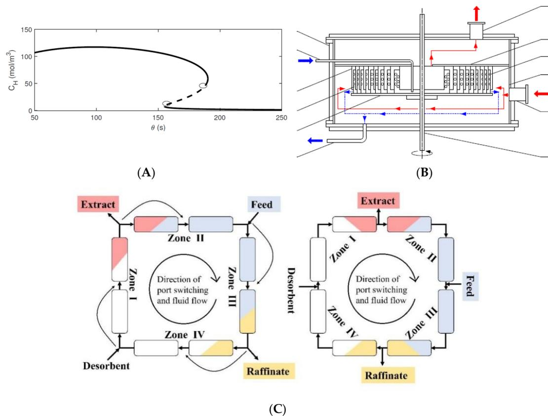
**Figure 3.** (A) Variations in hydrogen concentration with residence time in a membrane reactor [3]. (B) Diagram of a rotating zigzag bed [4]. (C) Simulated moving bed reactor [5].
