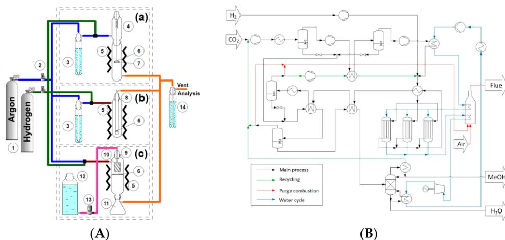
**Figure 6.** (A) Experimental setup of the catalytic decomposition of chlorinated hydrocarbons: (a–c), reactors (b); 1 gas cylinders; 2 flow mass controllers; 3 saturator; 4 quartz reactor; 5 heating zone; 6 catalyst sample; 7 foamed quartz basket; 8 lab flowthrough quartz reactor; 9 scaled-up quartz reactor; 10 evaporator; 11 carbon collector; 12 vessel; 13 pump; 14 alkali trap. [10]. (B) One-step process flowsheet [11].
