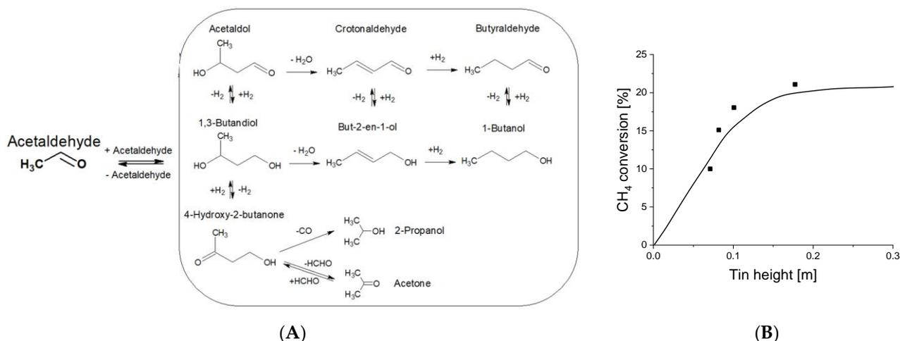
**Figure 2.** (A) Detailed reaction scheme of acetaldehyde condensation [1]. (B)  $\text{CH}_4$  conversion versus reactors’ axial coordinates for 6.0 cm ID reactor [2].
