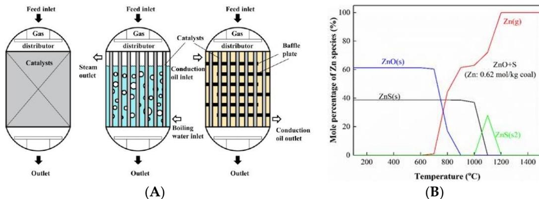
**Figure 5.** (A) Different industrial tubular reactors modeled in the work conducted by Huang et al. [8]. (B) Thermodynamic equilibrium distribution distributions of Zn when S and Zn coexist in the coal [9].
