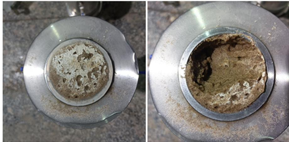
**Figure 11.** The plugging of the surface of the quartz-sand-packed layer by a mud cake (Scheme S4).
