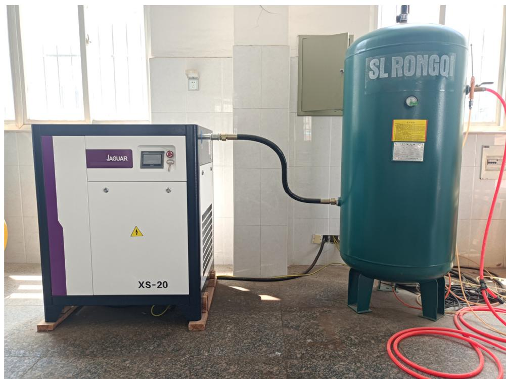
Figure 2. Photograph of the screw air compressor and air tank.
