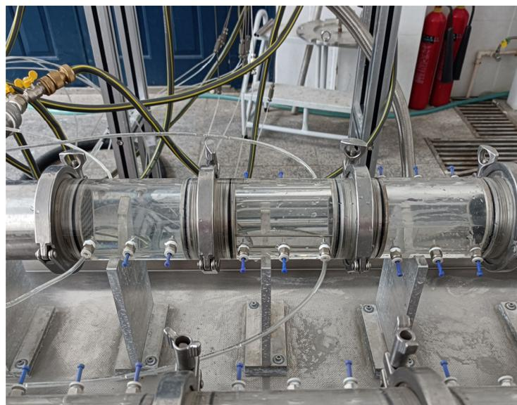
Figure 16. Gas-water mixed flow through the ceramic-particle-packed layer (Scheme S5).
