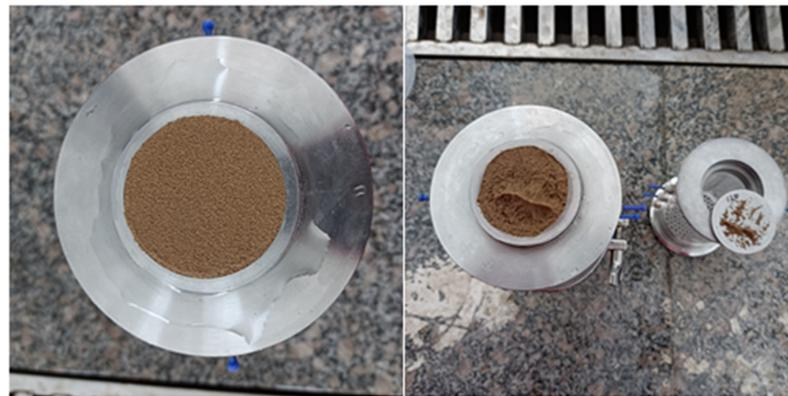
Figure 15. Surfaces of the ceramic-particle-packed layer before (left) and after (right) experiments (Scheme S5).
