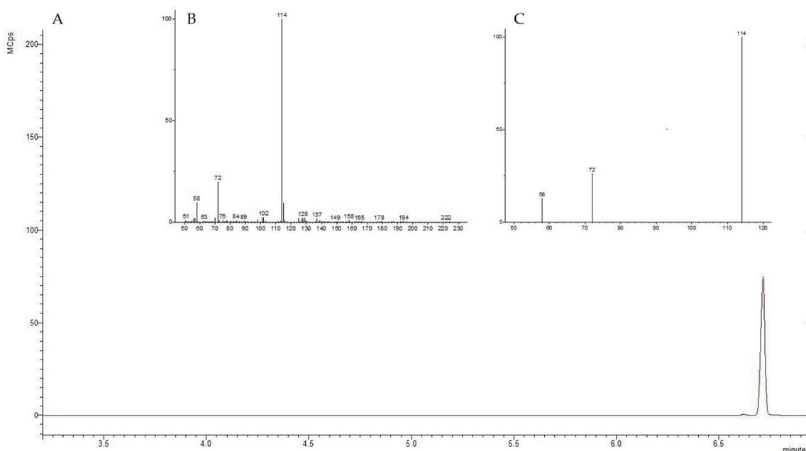
**Figure 4.** GC-MS chromatogram of the standard solution of 10 mg/mL sibutramine hydrochloride (A) according to MS spectrum in full scan (B) and SIM mode (C) with a retention time of 6.71 min.
