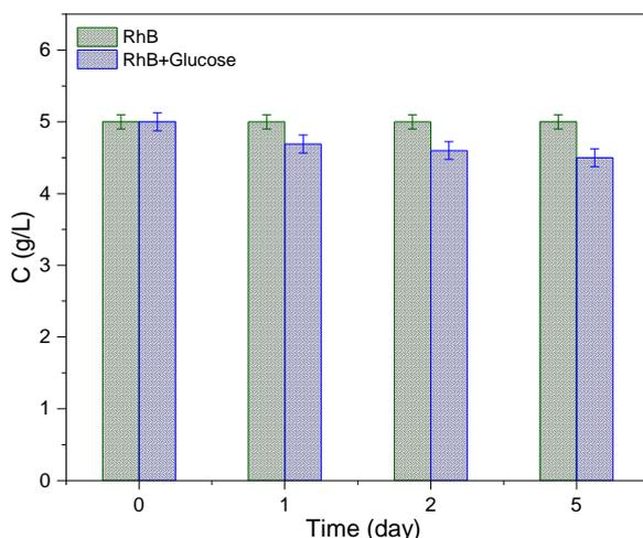
**Figure 6.** Assessment of concentration of RhB (C) in the presence of *S. cerevisiae* in mineral medium with and without glucose (Error < 5%).
