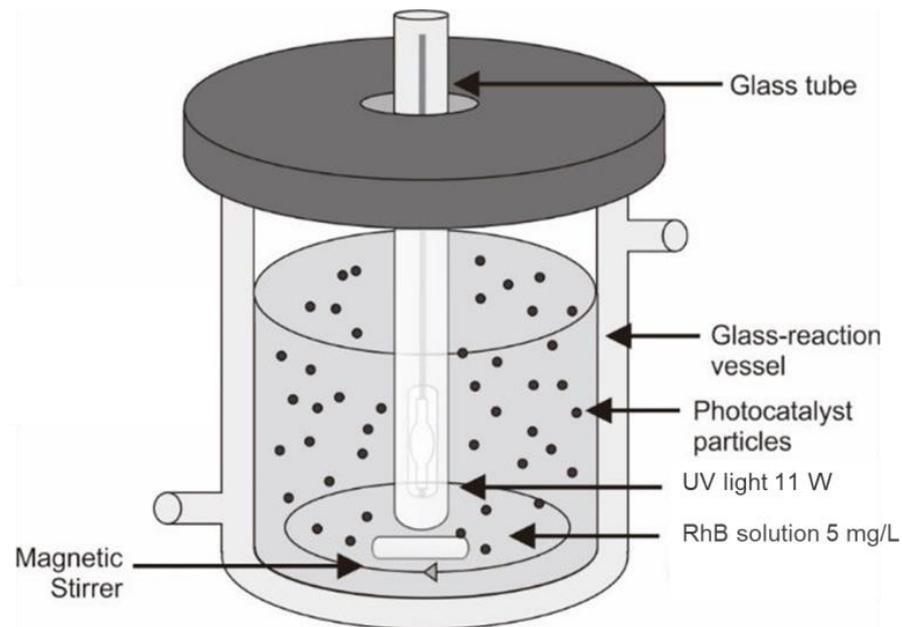
**Figure 2.** Photocatalytic reactor.
