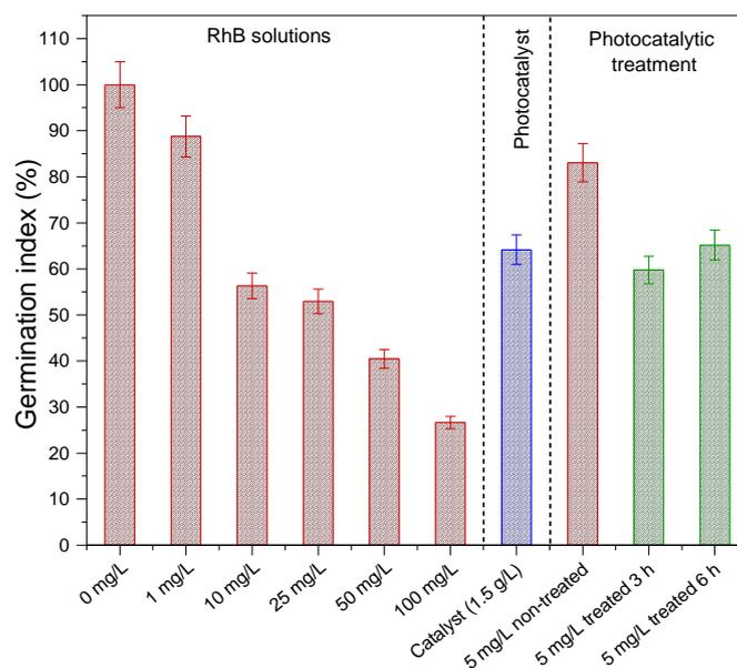
**Figure 8.** The phytotoxicity of the RhB solutions at different concentrations and the photocatalyst at  $1.5 \text{ g L}^{-1}$  and the solution after photocatalytic treatment at 3 and 6 h (Error < 5%).
