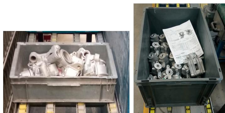
**Figure 5.** Transport containers used in the process of remanufacturing brake caliper bodies.
