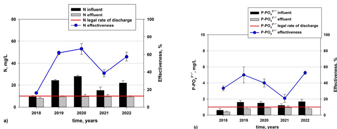
**Figure 6.** Total nitrogen (a) and phosphorous in phosphates (b) in wastewater in winter.
