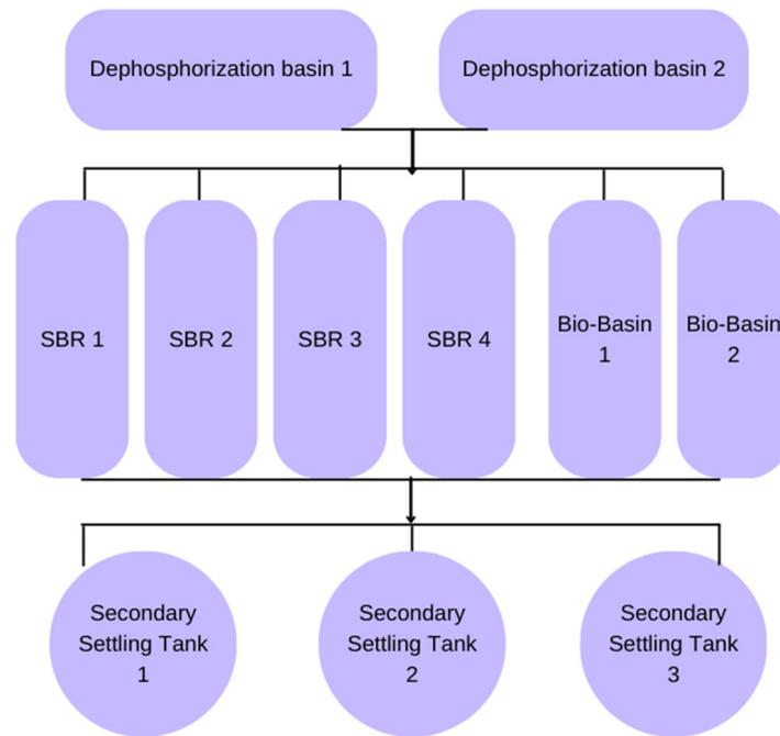
Figure 8. Simplified schema of biological treatment in WWTP Ravda during summer.
