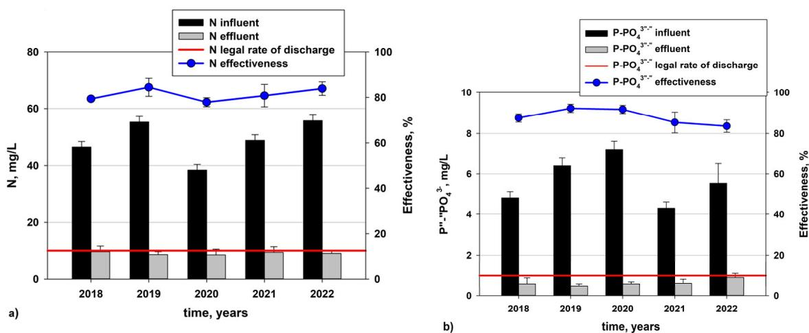
Figure 10. Total nitrogen (a) and phosphorous in phosphates (b) in wastewater in summer.
