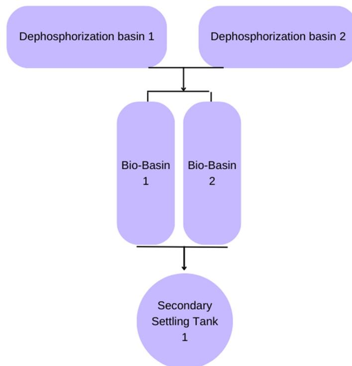
**Figure 4.** Simplified schema of biological treatment in WWTP Ravda during winter.
