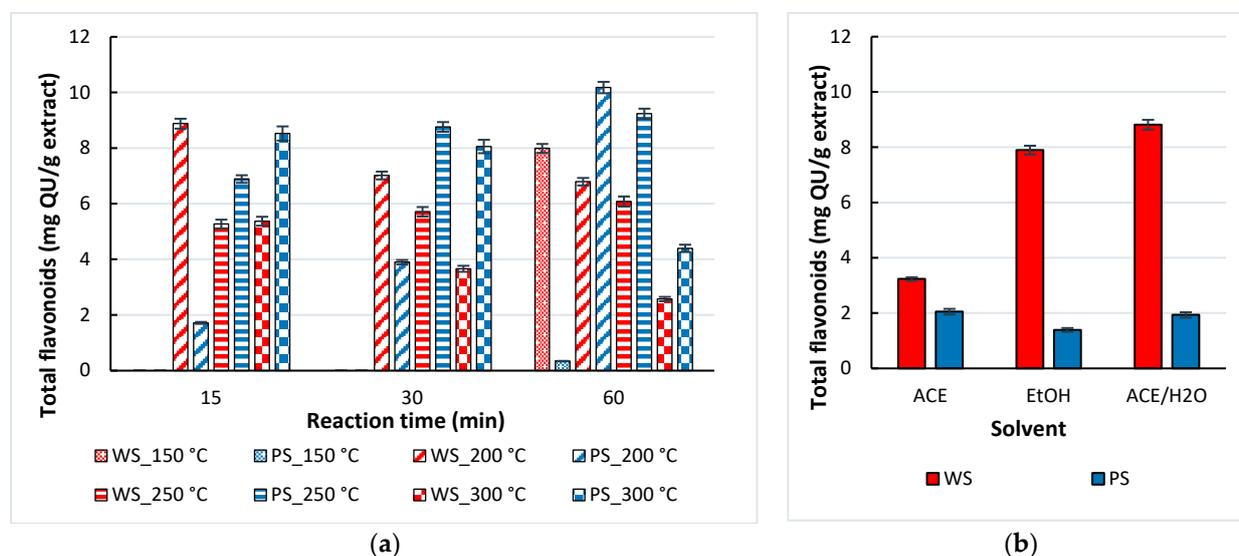
**Figure 6.** Content of total flavonoids in extracts of pistachio and walnut shells (PS-pistachio shells; WS-walnut shells) obtained via (a) SWE at various temperatures and reaction times and (b) conventional extraction with ACE-acetone, EtOH-ethanol, ACE/H<sub>2</sub>O-50% acetone.
