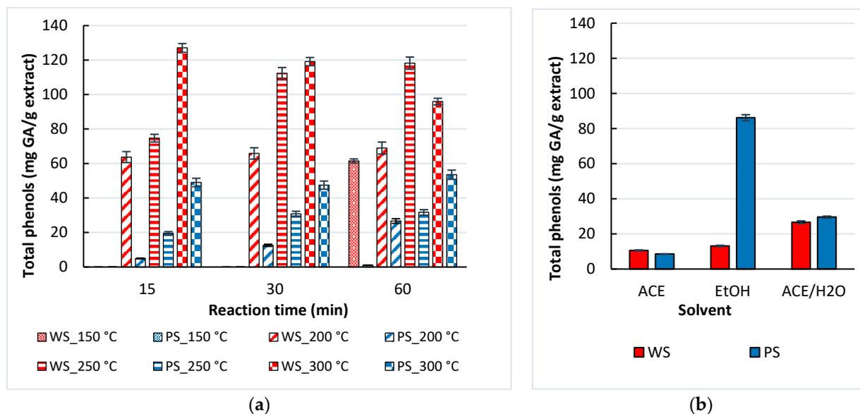
**Figure 5.** Content of total phenols in extracts of pistachio and walnut shells (PS-pistachio shells; WS-walnut shells) obtained via (a) SWE at various temperatures and reaction times and (b) conventional extraction with ACE-acetone, EtOH-ethanol, ACE/H<sub>2</sub>O-50% acetone.
