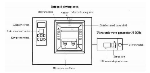
Figure 1. Direct-contact ultrasonic and far infrared combined drying equipment diagram.
