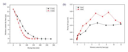
**Figure 4.** Drying curves and drying rate curves for different thickness. (**a**) Drying curves; (**b**) Drying rate curves.
