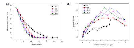
**Figure 3.** Drying curves and drying rate curves for different ultrasound frequencies. (**a**) Drying curves; (**b**) Drying rate curves.
