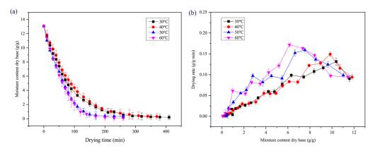
**Figure 2.** Drying curves and drying rate curves for different drying temperature. (**a**) Drying curves; (**b**) Drying rate curves.
