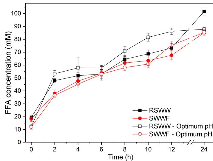
**Figure 2.** Influence of a pH adjustment on the enzymatic pretreatment.
