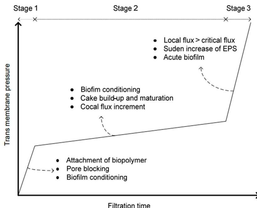
**Figure 6.** The mechanism and the occurrence of the TMP jump (stage 3) [52].
