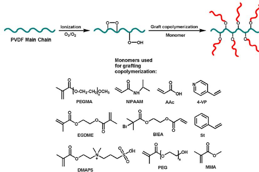
**Scheme 1.** Schematic illustration for the process of ozone pretreatment and subsequent graft copolymerization of PVDF with various monomers.
