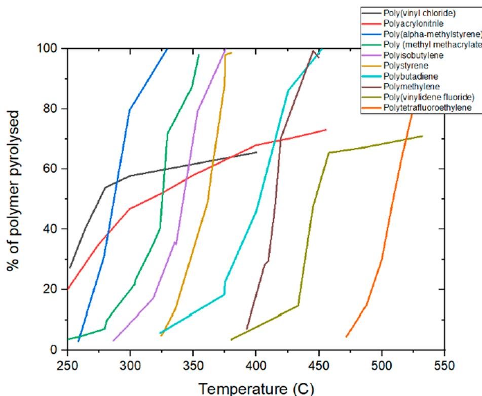
**Figure 1.** A graph illustrating the vaporization of several polymers during pyrolysis in a vacuum [10].
