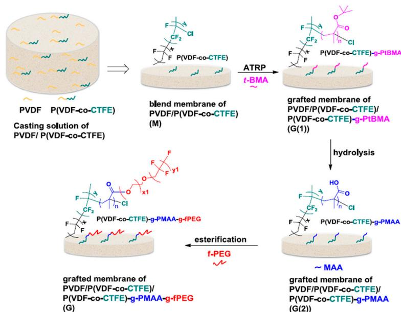
**Scheme 2.** Illustration of the grafting reactions on blend membrane's surface.
