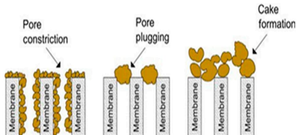
Figure 8. Pore constriction, pore plugging (clogging), and cake formation [58].
