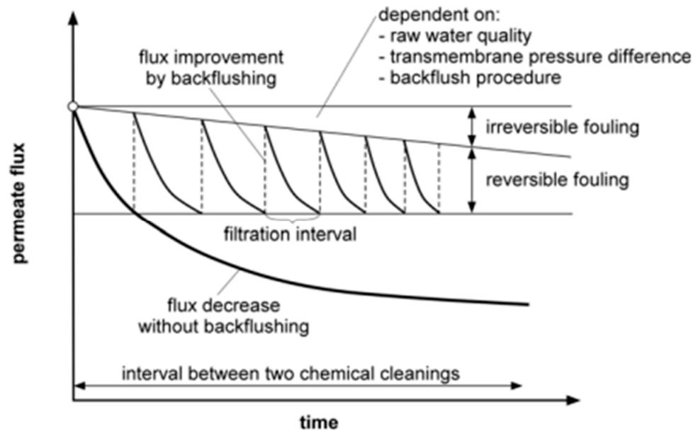
Figure 7. Reversible and irreversible foulings of the membrane [54].
