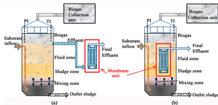
**Figure 3.** Diagrams for an immersed AnMBR (b) and a general side-stream AnMBR (a) are available in [32].
