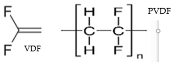
**Figure 2.** VDF and PVDF's structural formulae [20,21].
