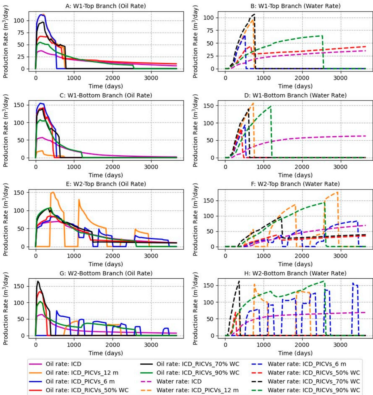
**Figure 16.** Comparative analysis of oil and water production rates across various branches in ICD-based completion scenarios.
