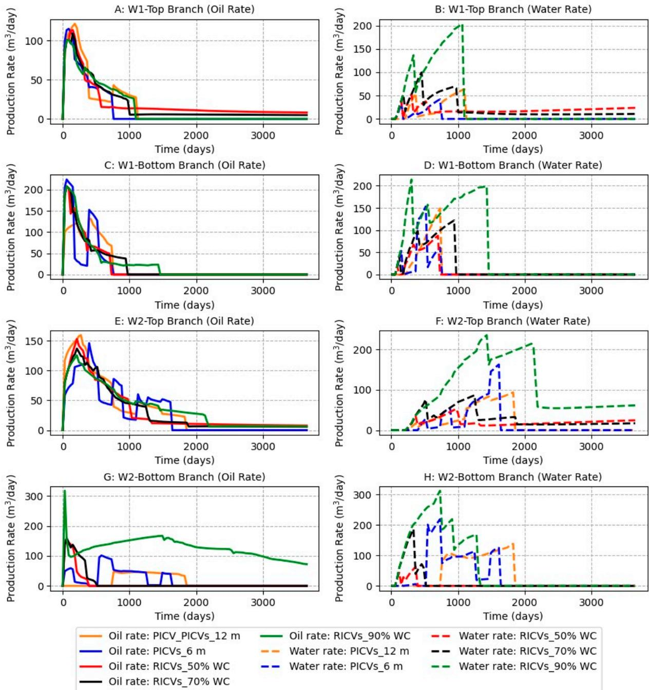
**Figure 18.** Comparative analysis of oil and water production rates across various branches in ICV-based completion scenarios.
