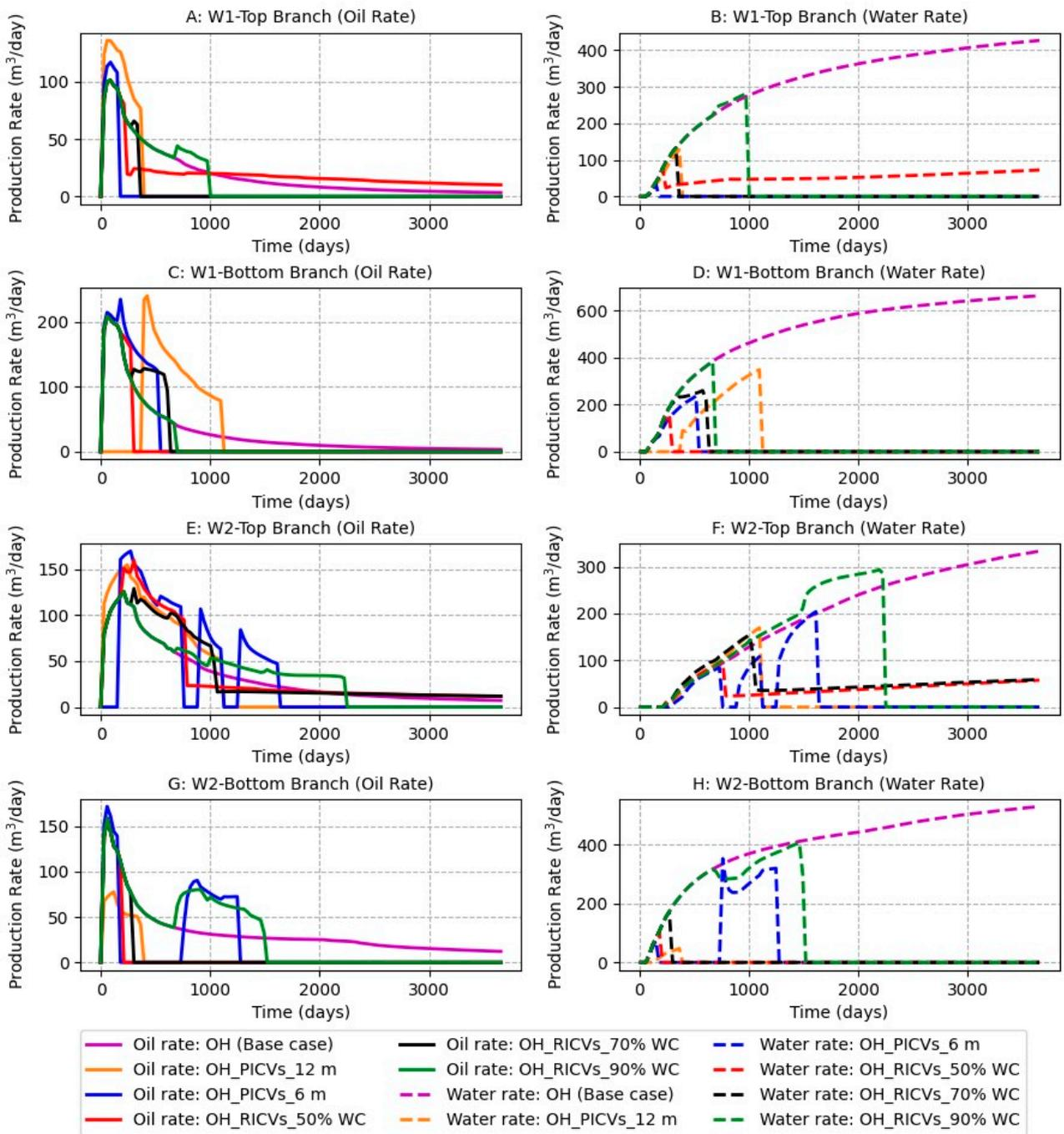
**Figure 15.** Comparative analysis of oil and water production rates across various branches in open hole-based completion scenarios.
