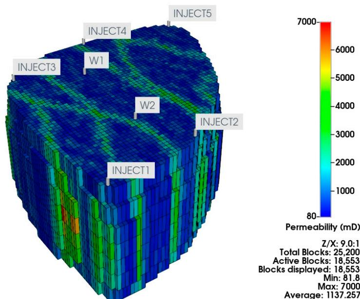
**Figure 7.** The egg reservoir model showing permeability distribution along the X-axis, as well as the names and positions of the wells.
