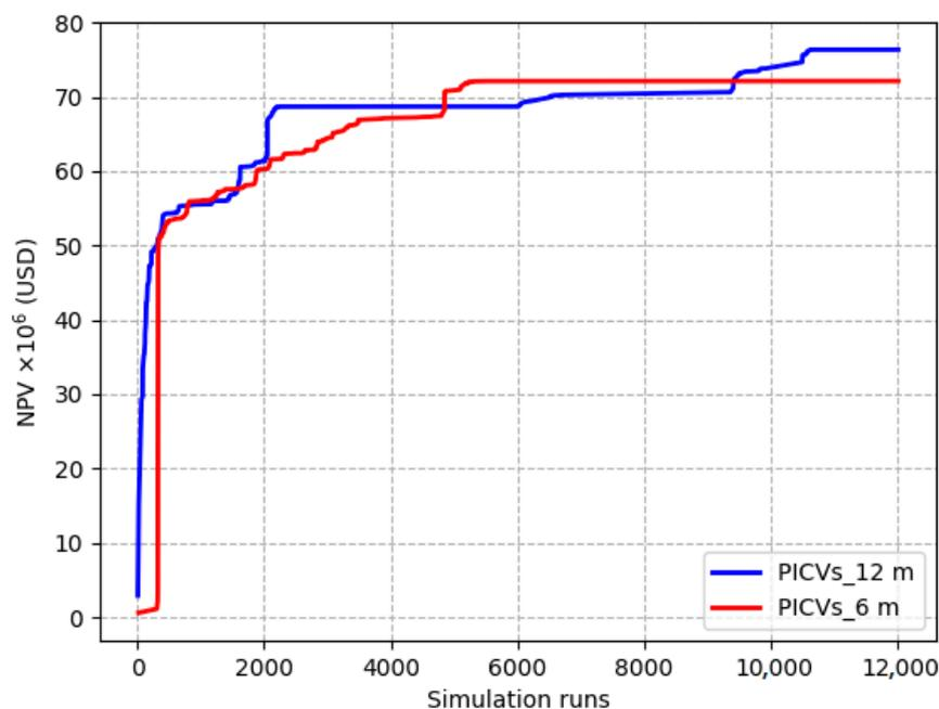
**Figure 11.** Extended simulation processes employing the GWO when the number of control variables experiences a substantial increase. The blue line represents the PICVs\_12 m case with 150 control variables, whereas the red line depicts the PICVs\_6 m case with 300 control variables.
