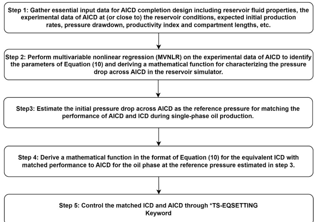
Figure 4. Workflow for matching ICD and AICD performance.
