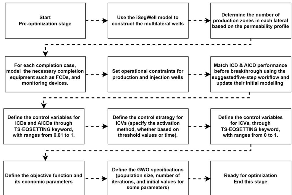
**Figure 5.** A pre-optimization stage framework: a detailed visualization of the key steps and processes leading to the preparation for dynamic optimization.
