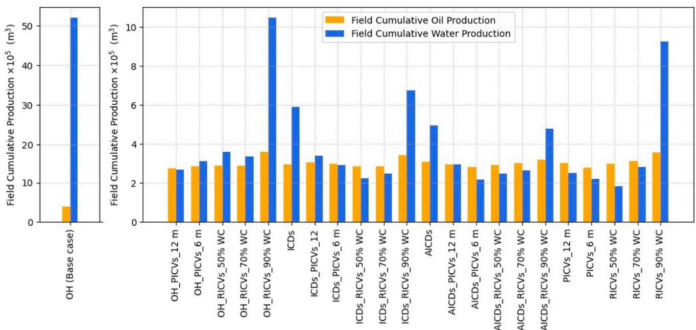
**Figure 12.** Field cumulative oil and water production for all completion cases.
