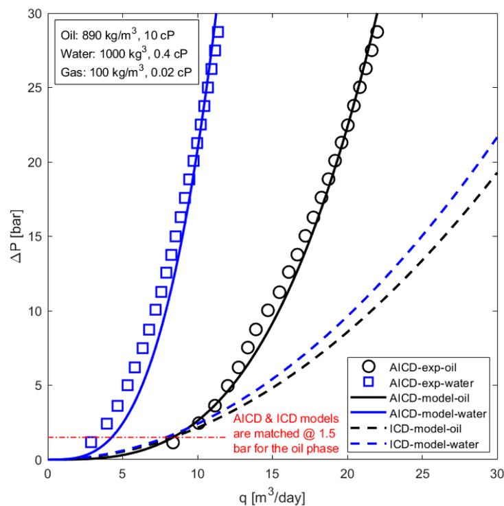
**Figure 9.** Comparison of AICD Experimental Data with AICD and ICD Mathematical Models, Demonstrating Matched Performance at the Reference Pressure.
