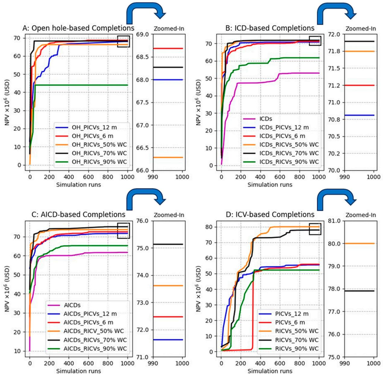
**Figure 10.** Optimization process using GWO for all 22 completion cases grouped into: (A) Open hole-based completion cases; (B) ICD-based completion cases; (C) AICD-based completion cases; (D) ICV-based completion cases.
