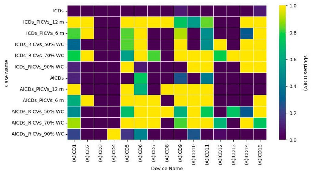
**Figure 14.** Normalized ICD and AICD settings (ranging from 0 to 1) for completion cases featuring passive and autonomous inflow control devices.
