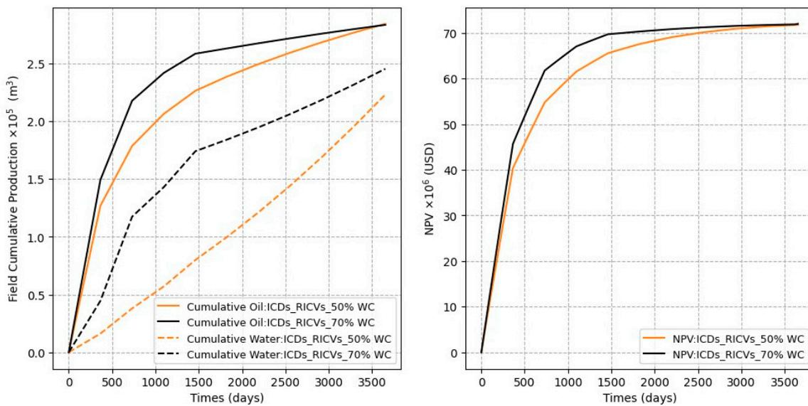
**Figure 13.** Comparison between ICDs\_RICVs\_50% WC and ICDs\_RICVs\_70% WC cases in terms of cumulative oil and water production (left) and NPVs (right).
