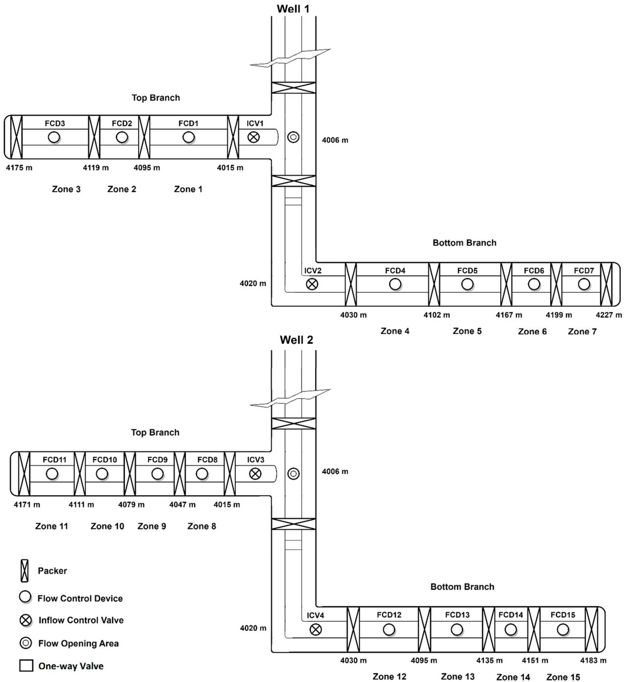
**Figure 8.** Completion schematics for production wells W1 (top) and W2 (bottom) in cases involving the use of multiple flow control devices (FCD here refers to either ICD or AICD depending on the case).
