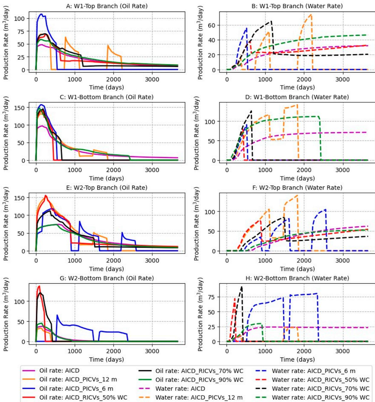
**Figure 17.** Comparative analysis of oil and water production rates across various branches in AICD-based completion scenarios.
