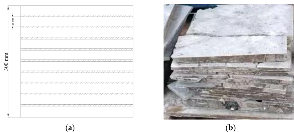
Figure 5. (a) Cutting schematic; (b) slices cut from the carbonate rock specimens.
