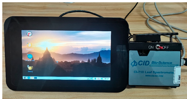
Figure 13. Hand-held VIS/NIR spectroscopy system designed for on-site prediction of chlorophyll and water content in maize leaves, consisting of a CI-710 spectrometer, Raspberry Pi 4B, and a 7-inch touchscreen.
