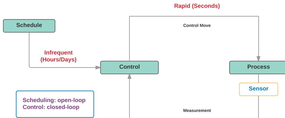
**Figure 1.** Phase 1: Open-loop scheduling determined once per day with no consideration of process dynamics. Closed-loop control implemented to follow the schedule.
