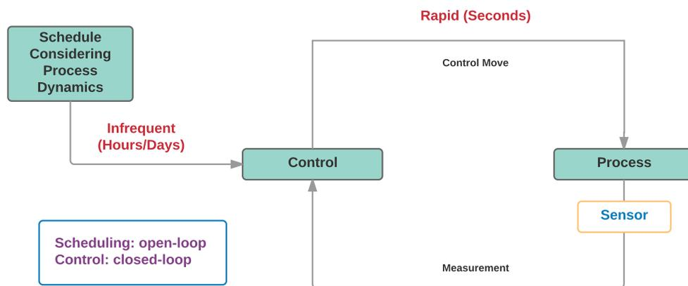
**Figure 3.** Phase 3: Open-loop scheduling determined once per day with consideration of process dynamics and control structure in the form of grade transition information. Closed-loop control implemented to follow the schedule.
