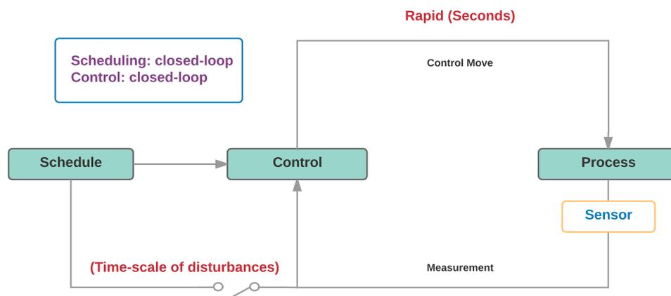
**Figure 2.** Phase 2: Dual-loop segregated scheduling and control. Scheduling is recalculated reactively in the presence of process disturbances above a threshold or updated market conditions. Closed-loop control implements the schedule in the absence of disturbances.
