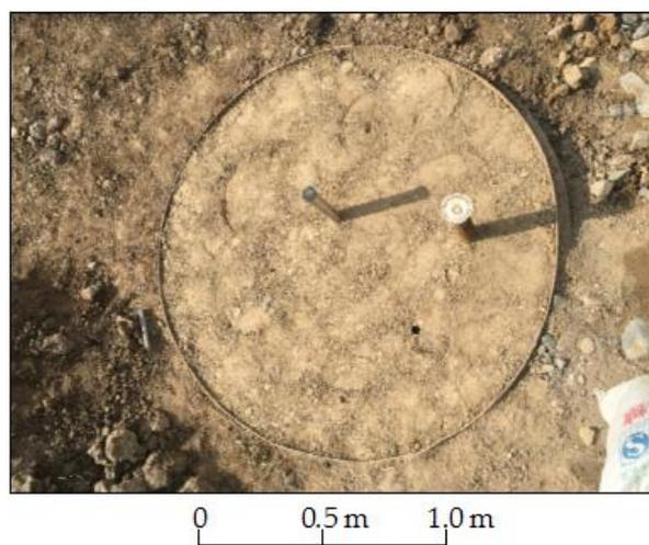
Figure 6. Reclaimed soil after one-compaction test barrel.
