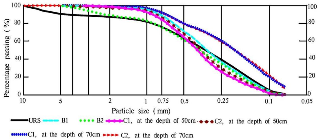
**Figure 16.** Accumulative curve of particle gradation of soil at the sampling depths of 50 cm and 70 cm.
