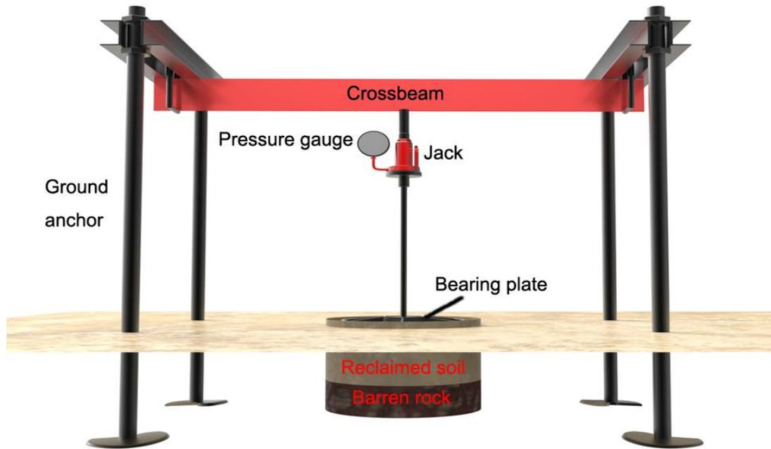
Figure 7. Illustration of the setup for plate load test.
