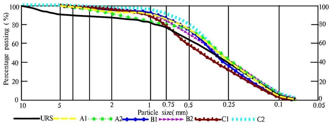
Figure 14. Accumulative curve of particle gradation of soil at the sampling depth of 10 cm.
