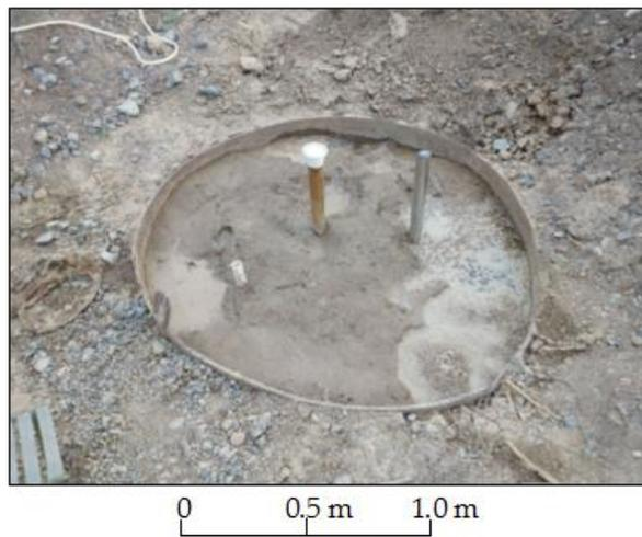
Figure 8. Uncompact reclaimed soil test barrel after irrigation.
