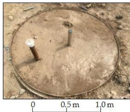
Figure 9. One-compaction reclaimed soil test barrel after irrigation.
