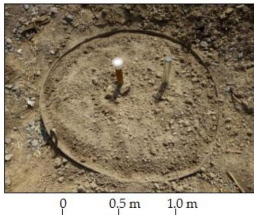
Figure 5. Uncompact reclaimed soil test barrel.
