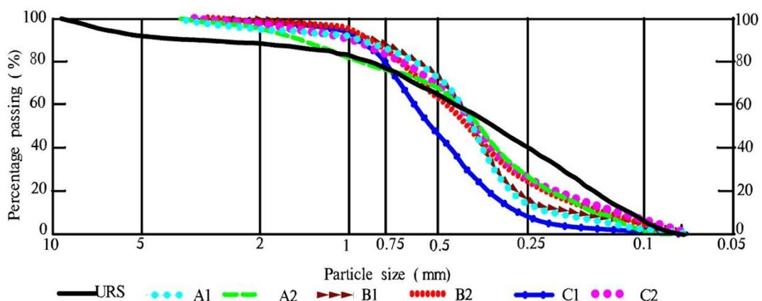
Figure 15. Accumulative curve of particle gradation of soil at the sampling depth of 30 cm.
