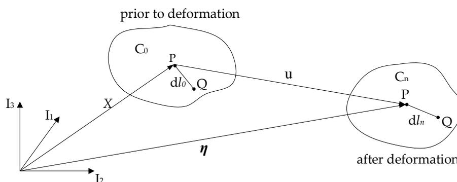
Figure 7. The particle motion during deformation.
