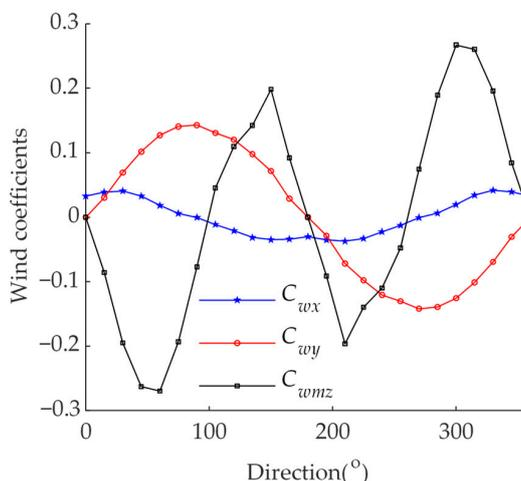
Figure 5. The wind coefficients for HYSY201.
