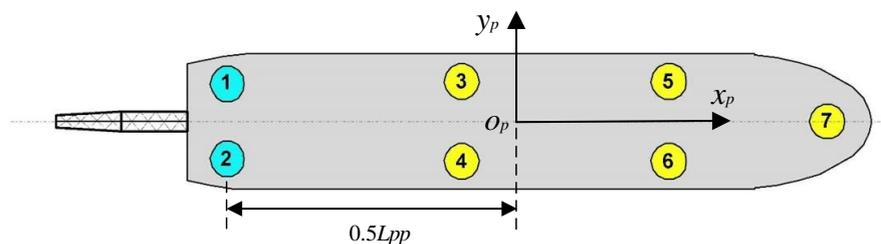
Figure 6. The arrangement and position of the HYSY201 thrusters.
