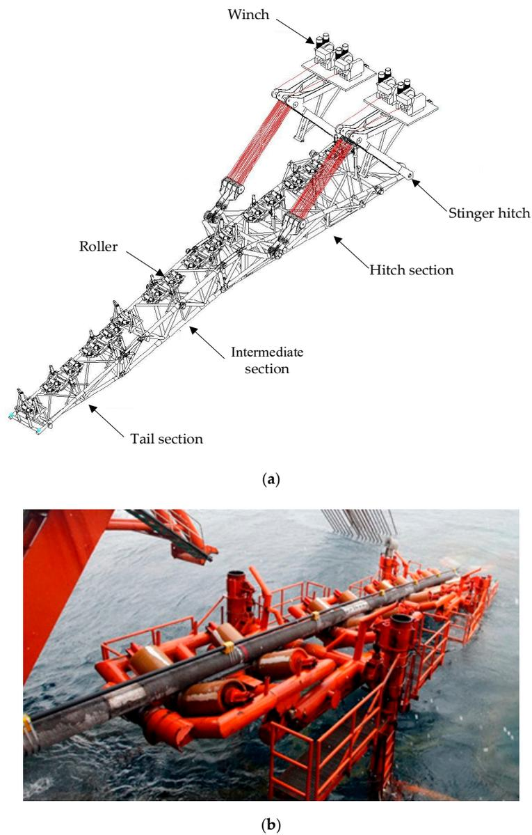
**Figure 8.** Stinger for S-laying operations: (a) articulated stinger of the HYSY201 and (b) the pipeline in contact with the stinger roller.
