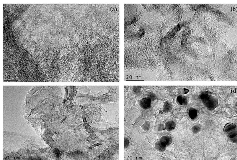
**Figure 2.** TEM images of carbonized chars with different amounts of FeCl<sub>3</sub> additive (a) C-HLH-5, (b) C-1FeHLH-5, (c) C-2FeHLH-5, and (d) C-3FeHLH-5.
