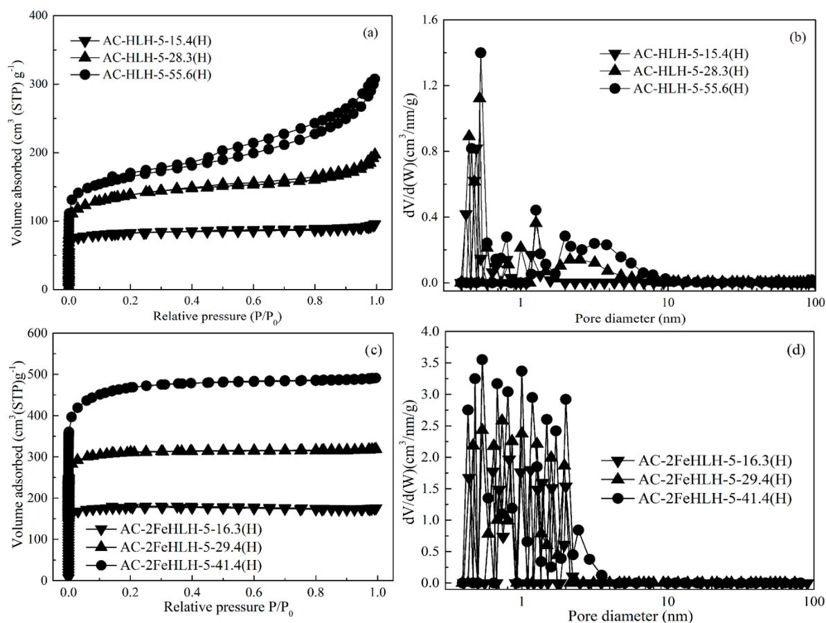
**Figure 6.** (a) N<sub>2</sub> adsorption isotherms and (b) pore-size distributions of AC-HLH-5 at different burn offs during activation; (c) N<sub>2</sub> adsorption isotherms and (d) pore-size distributions of AC-2FeHLH-5 at different burn offs during activation.
