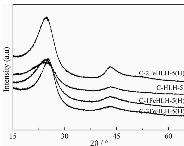
**Figure 4.** XRD profiles of carbonized chars with different amounts of FeCl<sub>3</sub> additive.
