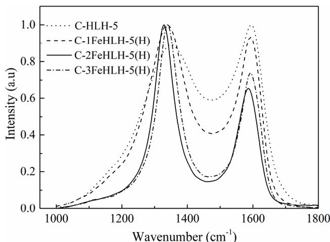
**Figure 3.** Raman spectra of carbonized chars with different amounts of  $FeCl_3$  additive.
