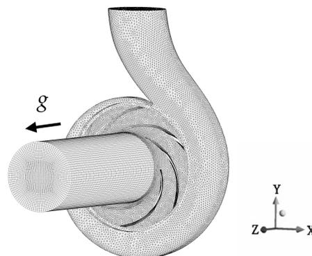
**Figure 2.** Computational domain and grids.  $g$  = gravitational acceleration.
