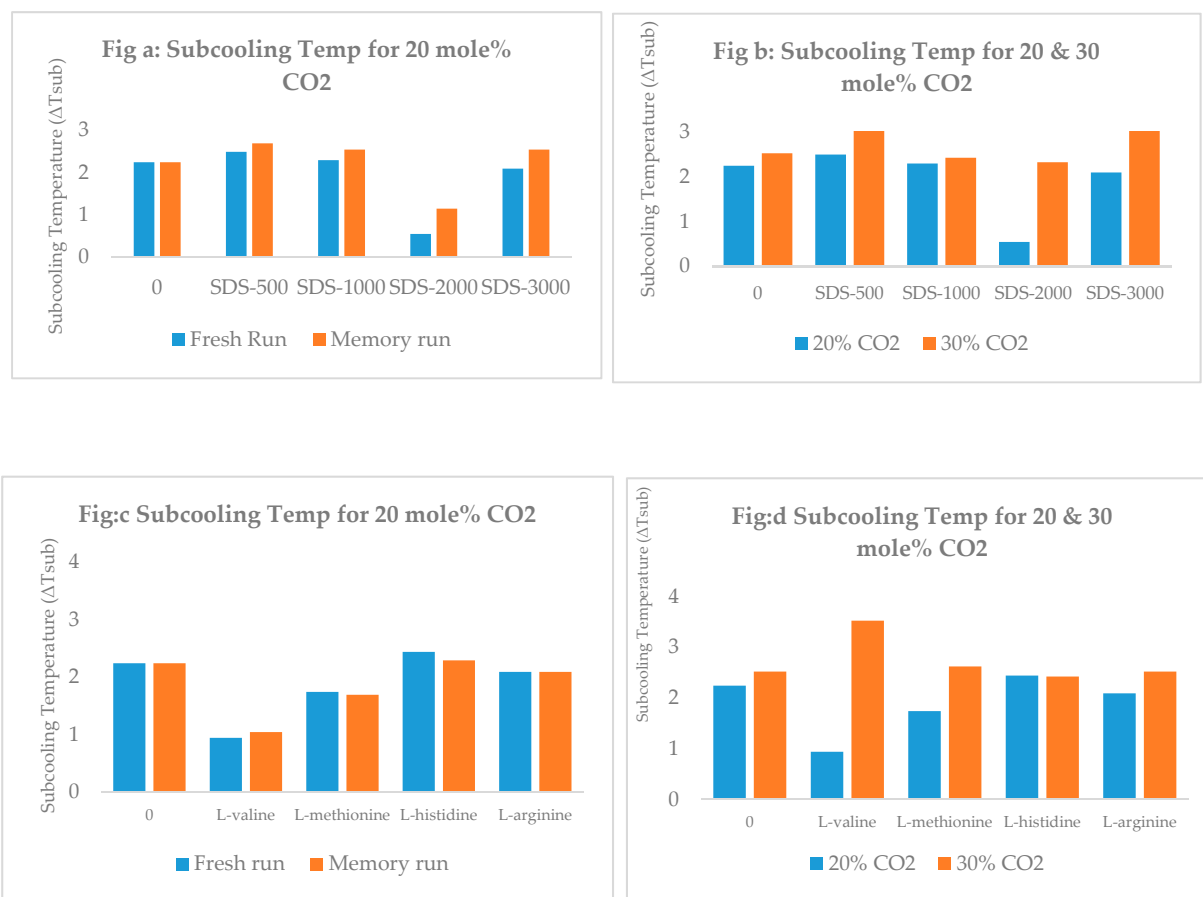
Figure 4. Subcooling kinetics in presence of amino acids and surfactant. Subcooling temperatures at the onset of the flue gas hydrate formation with amino acids and surfactant. (a) Subcooling temperature for 20% mole \text{CO}_2 for sodium dodecyl sulfate (SDS) at different concentration (fresh and memory). (b) Subcooling temperature for 20 and 30 mole% \text{CO}_2 for SDS at different concentration (fresh). (c) Subcooling temperature for 20% mole \text{CO}_2 for amino acids at different concentration (fresh and memory). (d) Subcooling temperature for 20 and 30 mole% \text{CO}_2 for amino acids at different concentration (fresh).
