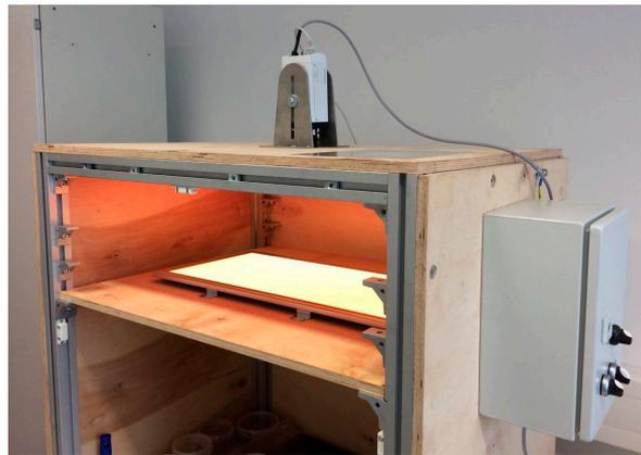
**Figure 2.** Experimental setup for fuel photography at FAU-EVT (with removed front cover).
