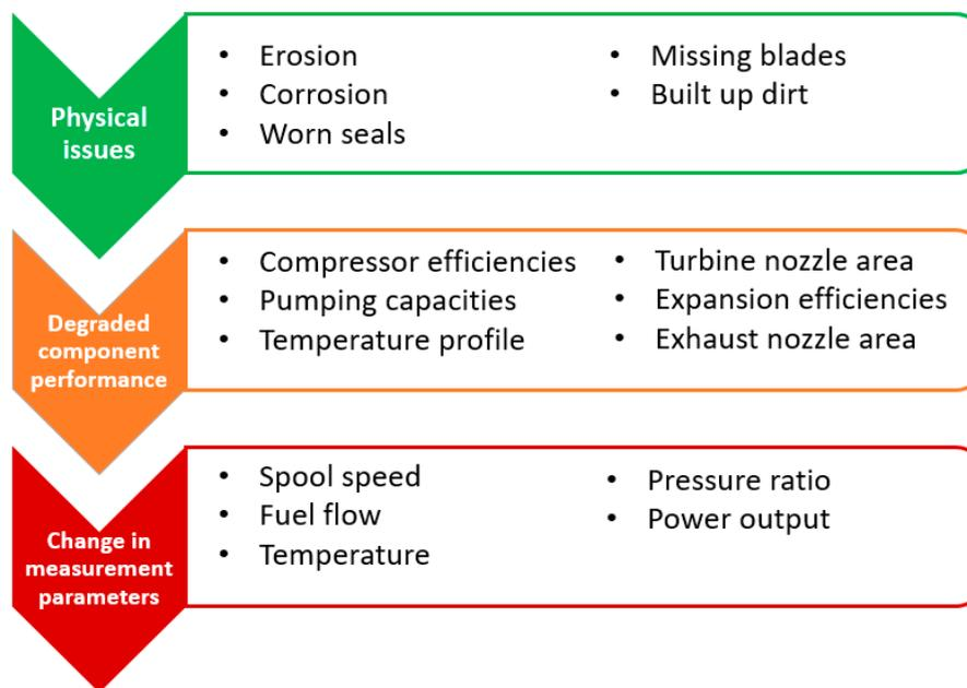
Figure 3. Gas turbines (GTEs) fault diagnostics approach [20,26].
