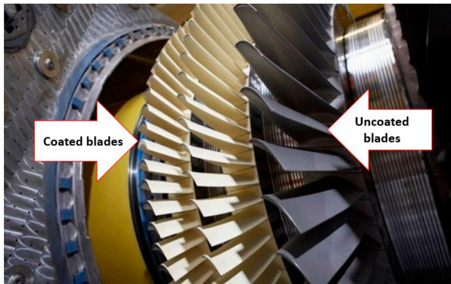
Figure 17. Coated and uncoated compressor blades [129].
