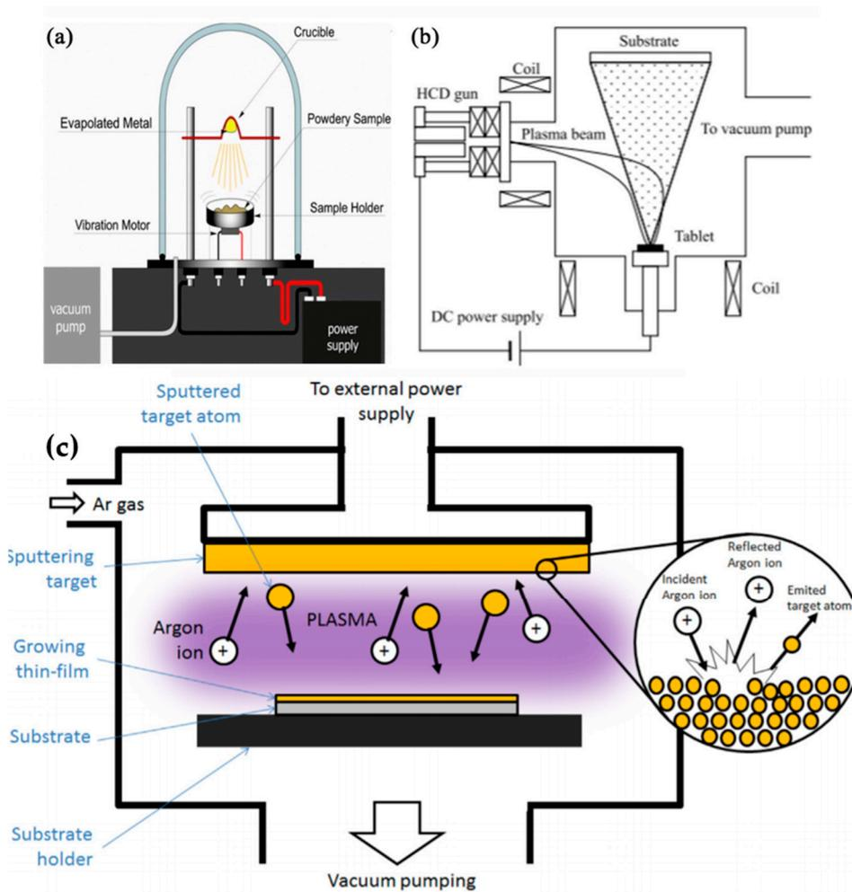
**Figure 18.** The three most common PVD coating approaches, where (a) shows a vacuum deposition process [158], (b) illustrates a schematic drawing of the ion-plating method [159], and (c) demonstrates the physical sputtering processes [160]. Reproduced with permission from [160]. Elsevier, 2015.
