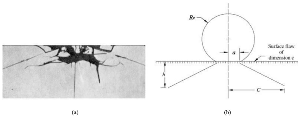
**Figure 11.** SPE on a brittle material, where (a) illustrates the cracks formed on the surface after the solid particles impact, and (b) shows the cracking propagation. Reproduced with permission from [69]. Springer Nature, 2001.
