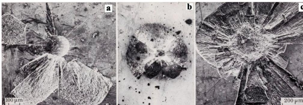
**Figure 13.** Common impact deformation patterns noticed in the brittle material as a plastic reaction regime, where (a) shows the radial cracking that generated from the central impression and material
