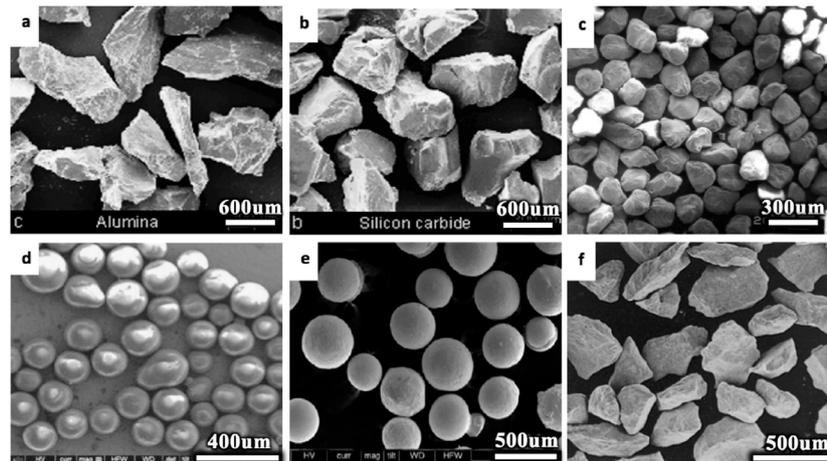
**Figure 16.** Particle materials and shapes used in experimental studies: (a) alumina [88], (b) silicon carbide [88], (c) quartz [89], (d) glass beads [90], (e) steel round grit [91], and (f) tungsten carbide [92]. Reproduced with permission from [82–86]. Elsevier, 2008, 2001, 2015, 2013, and 1999, respectively.
