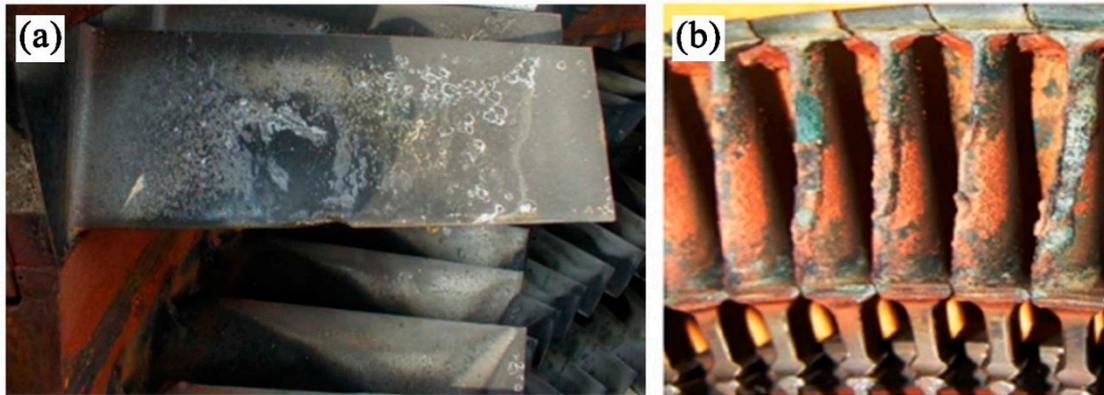
**Figure 1.** Illustration of degradation damages on the surface of: (a) compressor blades, and (b) turbine blades. Reproduced with permission from [17]. ASME, 2006.
