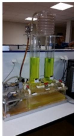
**Figure 14.** Two-tank system.
