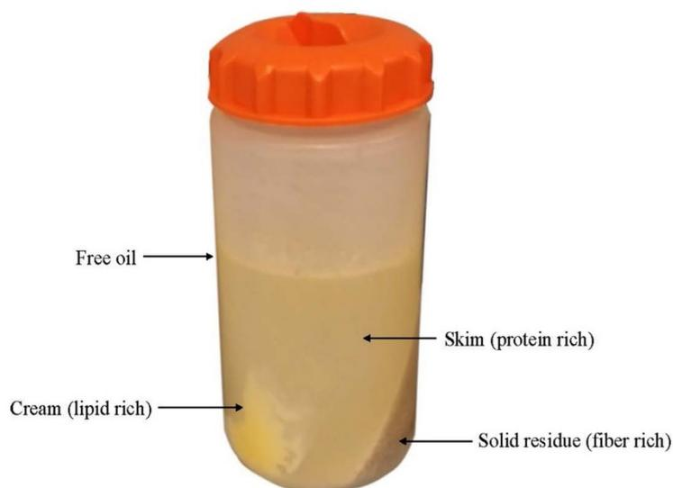
**Figure 3.** Image of partitioning in aqueous extraction slurry after centrifugation.
