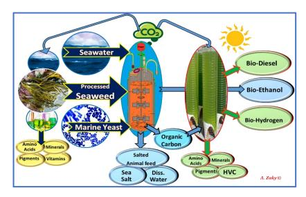
Figure 6. Coastal integrated marine biorefinery (CIMB) system (Route 2).
