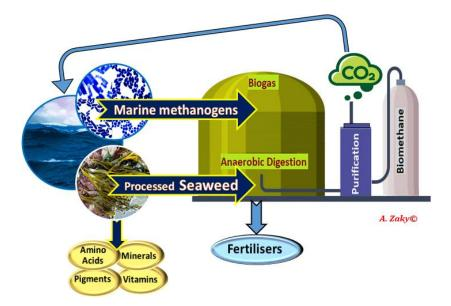
Figure 4. CMB system for the production of biogas (Route 2).
