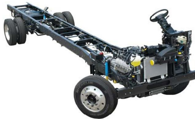
**Figure 1.** A ladder chassis frame (truck) view [6].
