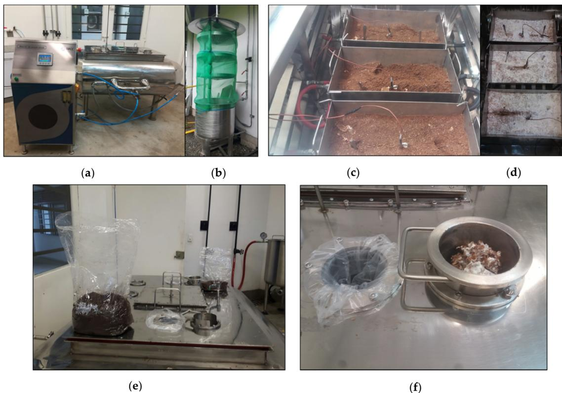
**Figure 1.** Details of the fixed-bed pilot-scale bioreactor. (a) Body of the bioreactor with panel for temperature control and air supply device. (b) Perforated-plate cooling tower for water recycling. (c) Bioreactor boxes loaded with 10 kg inoculated substrate each. (d). Boxes with colonized substrate. (e) Loaded bioreactor under operation. (f) Sampler for follow-up of the fermentation process.
