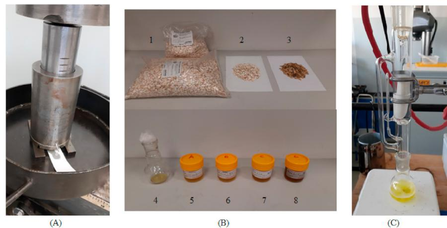
**Figure 1.** Uniaxial compression process of pumpkin seeds: (A) Oil point identification and oil extraction; (B–1) Bulk pumpkin seeds, (B–2) Measured sample before oil extraction, (B–3) Sample seedcake after oil extraction, (B–4) Sample oil through Soxhlet extraction, (B–5) Compressed oil at 20 °C (Control), (B–6) at 40 °C; (B–7) at 60 °C, (B–8) at 80 °C, and Soxhlet extraction setup (C).
